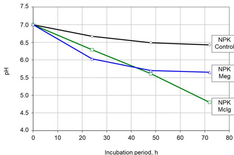
**Figure 2.** The influence of the bacterial inoculant on the temporal variation of solution pH.
