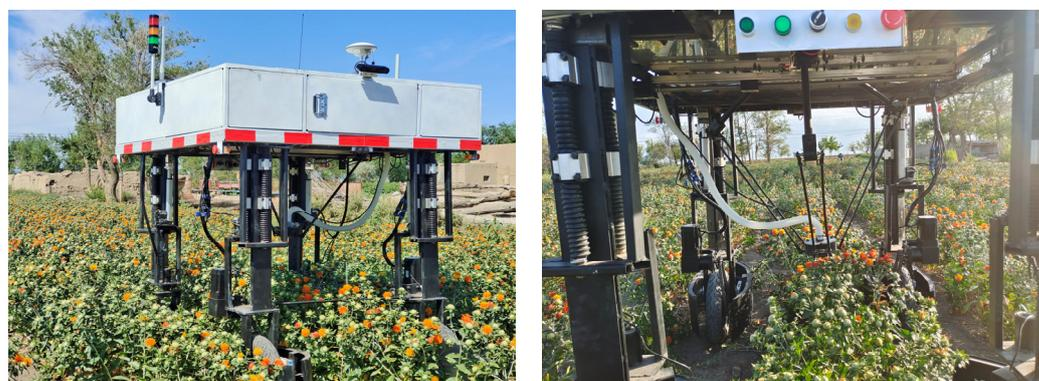
Figure 15. Safflower-picking robot field experiment.
