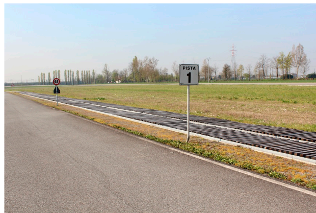
Figure 3. The International Standards Organization (ISO) 5008 100m smooth test track.
