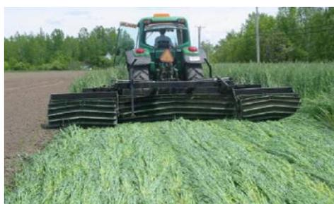
**Figure 1.** Adaptation of the roller-crimper by the Dewavrin brothers in Les Cèdres, Québec. Reproduced with permission from Estevez, 2008 [13]. Plans are available online for free [31].
