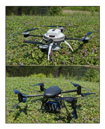
**Figure 5.** Two unmanned arial system (UAS) quadrocopters deployed by Nipissing University researchers for agricultural monitoring. The Aeryon Scout (Aeryon Labs Inc., Waterloo, ON, Canada) carries (top photo) an infrared ADC lite camera (Tetracam, Chatsworth, CA, USA), whereas the Dragan Flyer X-8 (Draganfly Innovations Inc., Saskatoon, SK, Canada) carries a Mini-MCA camera (Tetracam, Chatsworth, CA, USA).
