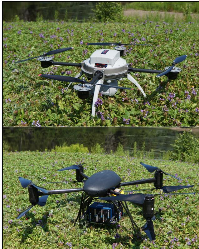
**Figure 5.** Two unmanned aerial system (UAS) quadcopters deployed by Nipissing University researchers for agricultural monitoring. The Aeryon Scout (Aeryon Labs Inc., Waterloo, ON, Canada) carries (top photo) an infrared ADC lite camera (Tetracam, Chatsworth, CA, USA), whereas the Draganfly X-8 (Draganfly Innovations Inc., Saskatoon, SK, Canada) carries a Mini-MCA camera (Tetracam, Chatsworth, CA, USA).
