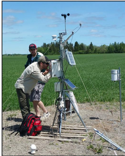
**Figure 1.** One of the many weather stations maintained for the *GeoVisage* system. This HOBO U30 station, located in Temiskaming Shores, has been actively collecting data since 3 July 2009.
