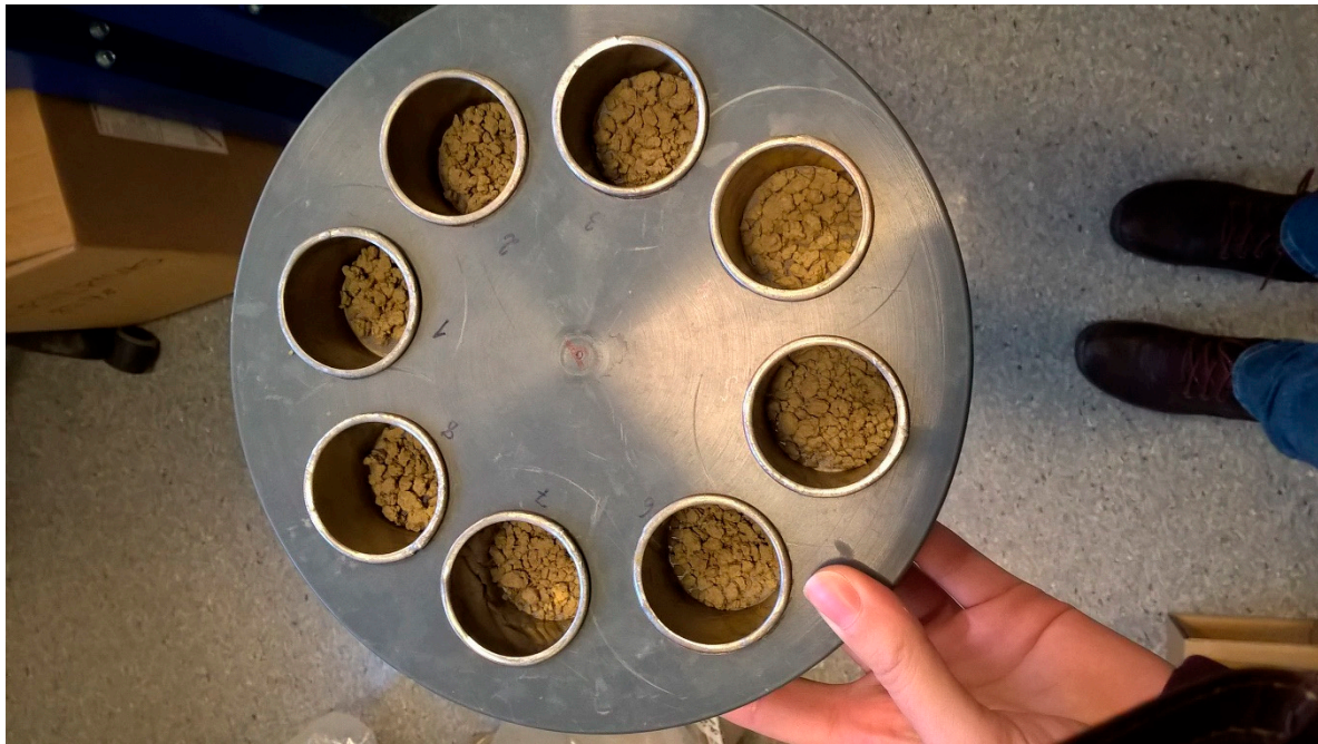
Fig. S5. Approximately 15 g of 2-6mm sized aggregates placed in small sieves prior to pre-wetting and wet sieving. Some of the aggregates were later found to be large biochar particles encrusted in thin films of clay.
