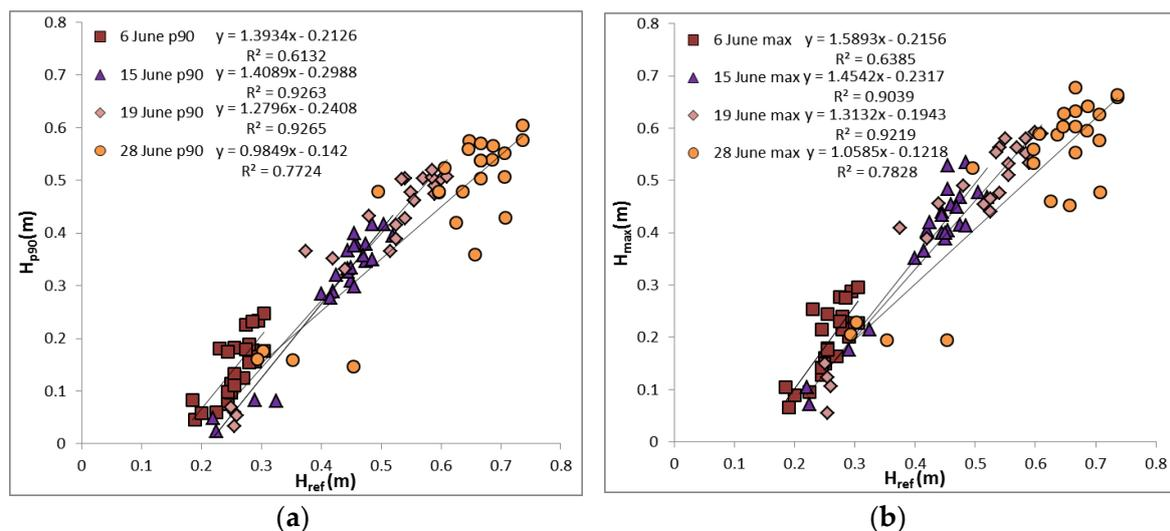
**Figure 5.** Simple linear regression of (a)  $H_{p90}$  and  $H_{ref}$  and (b)  $H_{max}$  and  $H_{ref}$  for different dates.  $H_{p90}$ : the 90th percentile value from the CHM;  $H_{max}$ : maximum value from the CHM; and  $H_{ref}$ : reference height measurement.
