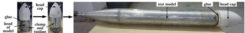
Figure 11. Test model with buffer head cap.
