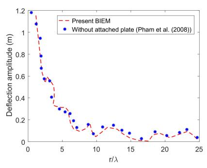
Figure 4. Comparison of deflection amplitude between BIEM and the result [28].
