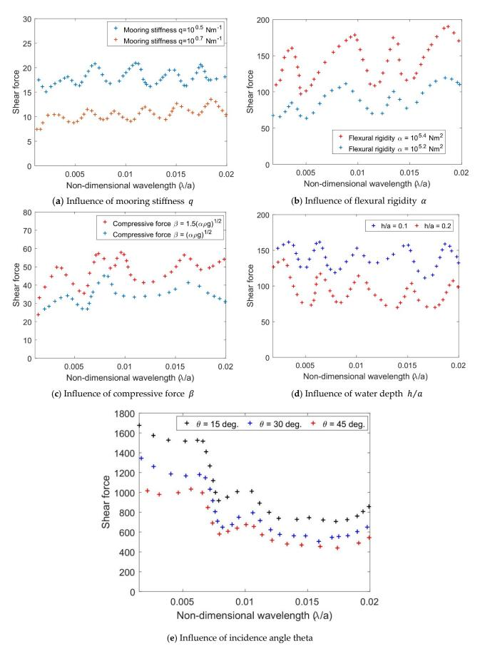
**Figure 6.** Variation in shear force on different q,  $\alpha$ ,  $\beta$ , and h/a versus  $\lambda/a$  with  $\alpha = 10^5$ ,  $\beta = 1.5\sqrt{EI\rho g}$ .
