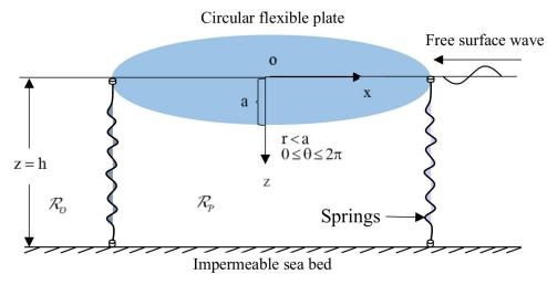
Figure 1. Hydroelastic model configuration.
