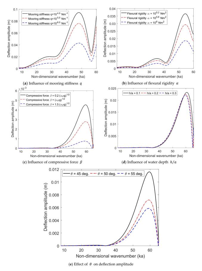
**Figure 8.** Variations in deflection amplitude on different q,  $\alpha$ ,  $\beta$ , and h/a versus  $\lambda/a$ .
