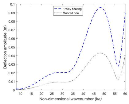
**Figure 5.** Comparison between freely floating and moored structures (spring stiffness  $q = 10^5 \text{ Nm}^{-1}$ ) with h/a = 0.5.
