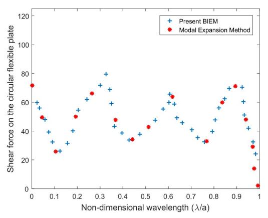
Figure 3. Comparison of shear force between BIEM and the result [24].
