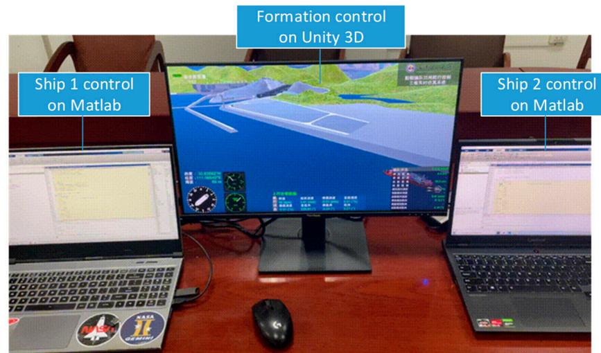
Figure 12. Vessel formation simulation system for lock waters.
