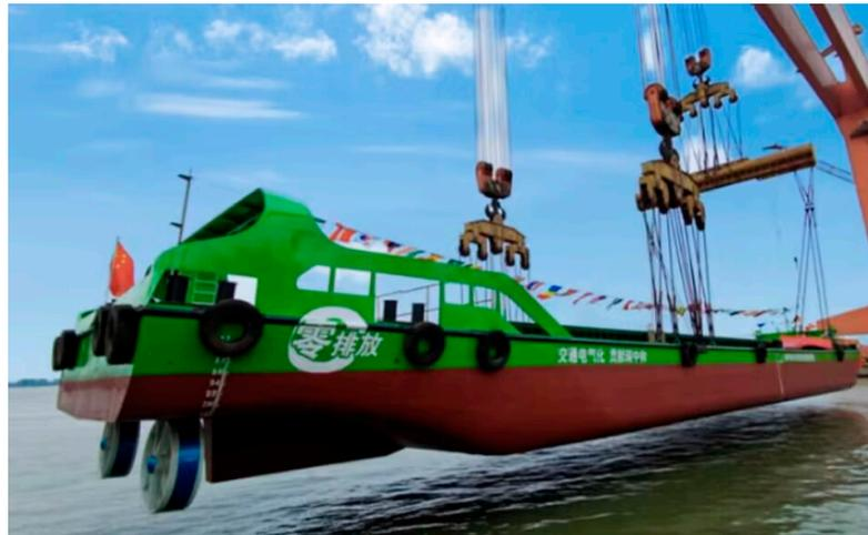
**Figure 6.** The 64 TEU battery-powered container ship Guochuang with zero emission.
