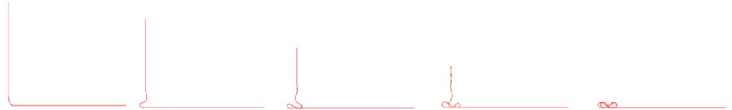
**Figure 3.** Configuration of a cable with the fast static equilibrium calculation method.
