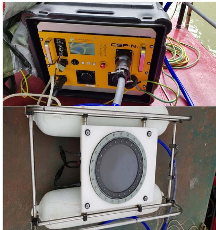
Figure 8. Parts of the recording system used for the survey: energy source (top) and Boomer plate (bottom).
