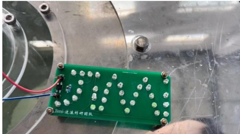
**Figure 24.** Prototype lights the LED lamp under the action of a regular wave with a height of 0.12 m and a period of 2.5 s.
