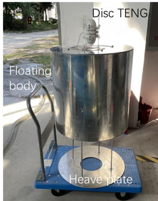
Figure 11. Physical picture of the center pipe wave energy triboelectric nanogenerator.
