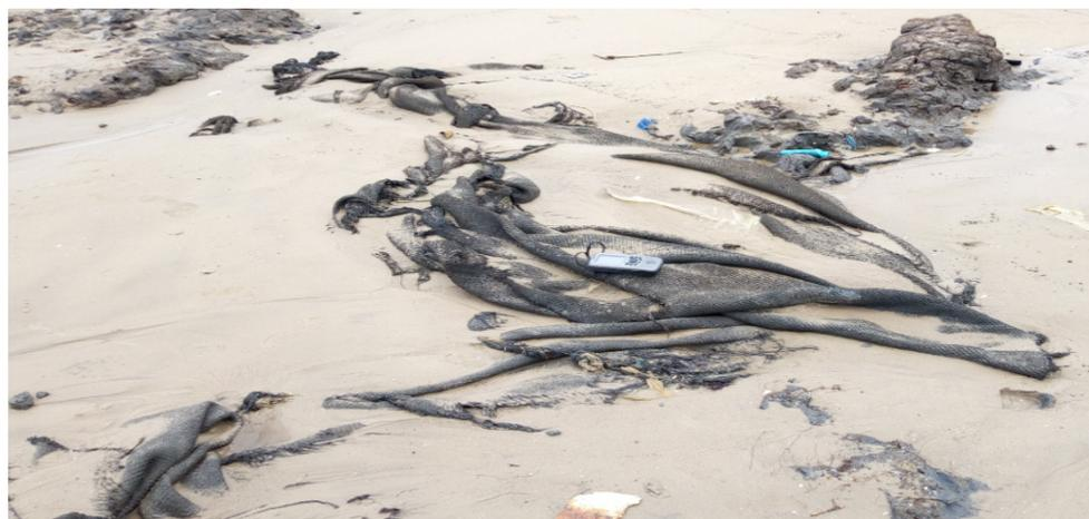
**Figure 2.** Failed jute tube on the sea shore of Ayetoro.
