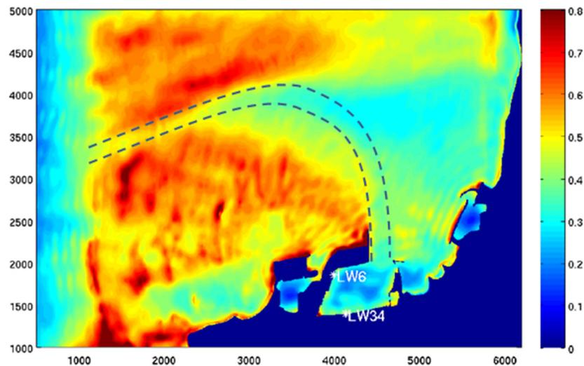
**Figure 5.** Example of FUNWAVE [31] long period wave significant wave height for an event on 2009-09-12. The boundary sea-swell  $H_s$  at  $T_p$  were 4.1 m and 17.3 s respectively. Units are in m. Figure courtesy Port of Geraldton, produced by MetOcean Solutions, with permission.
