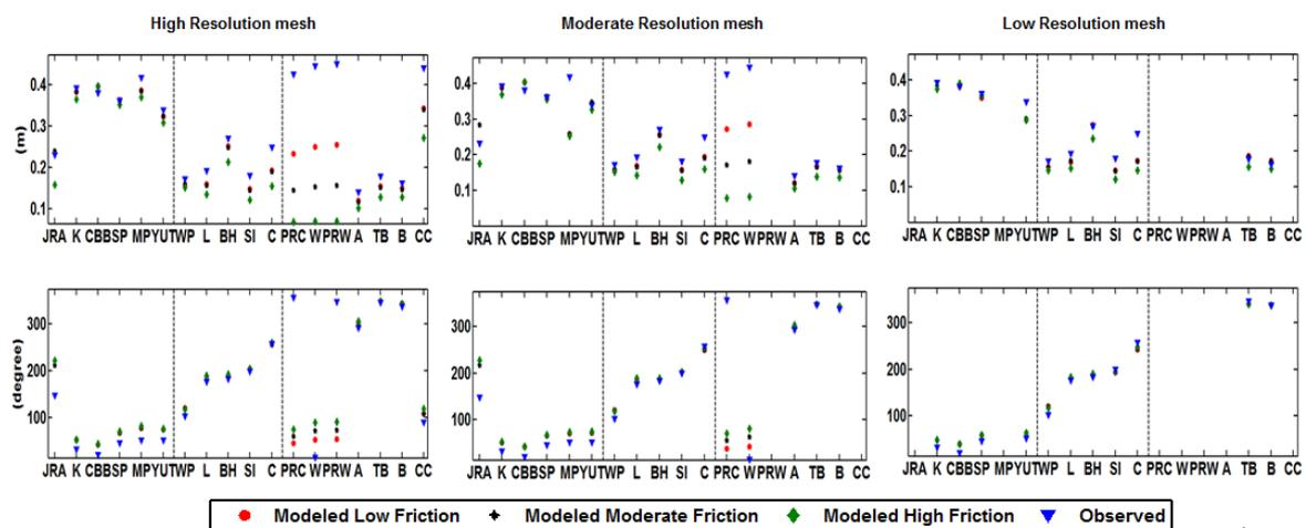
**Figure 6.** Observed and modeled amplitude and phase  $M_2$  constituent at those stations described in Table 4. The simulations were performed on three levels of roughness and three levels of resolution.
