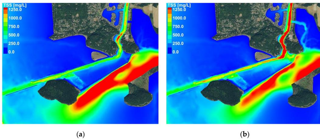
Figure 15. Time averaged total suspended sediment (TSS) distribution (20 days) for (a) baseline conditions and (b) McGlinn Causeway restoration, SCN-2.
