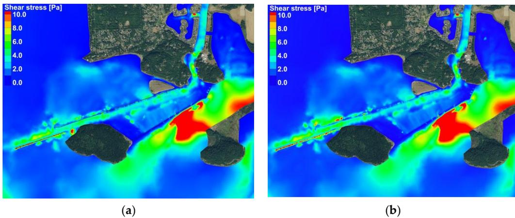
**Figure 11.** Time averaged bottom shear stress distribution (20 days) for (a) baseline conditions and (b) Jetty Repair Scenario, SCN-1.
