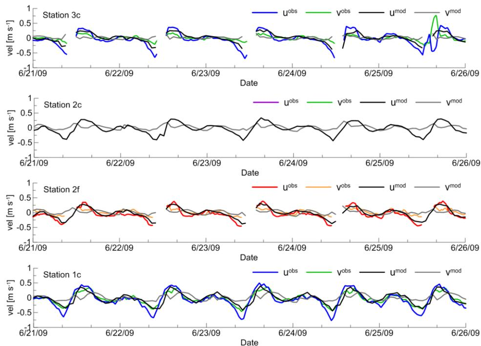
**Figure 5.** Comparison of bottom currents in Skagit tidal flats shown at stations 3c, 2c, 2f and 1c during June of 2009 as part of sediment model setup and calibration. ( $u^{obs}$  = observed east velocity component,  $v^{obs}$  = observed north velocity component,  $u^{mod}$  = modeled east velocity component and  $v^{mod}$  = modeled north velocity component).
