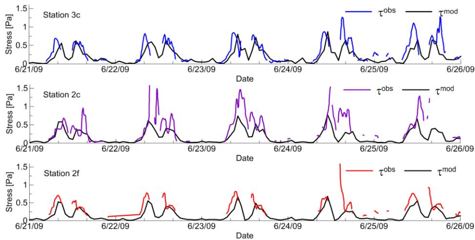
**Figure 6.** Comparison of observed bottom stress in Skagit tidal flats shown at stations 3c, 2c and 2f during June of 2009 as part of sediment model setup and calibration. ( $\tau^{\text{obs}}$  = observed bottom shear stress and  $\tau^{\text{mod}}$  = modeled bottom shear stress).
