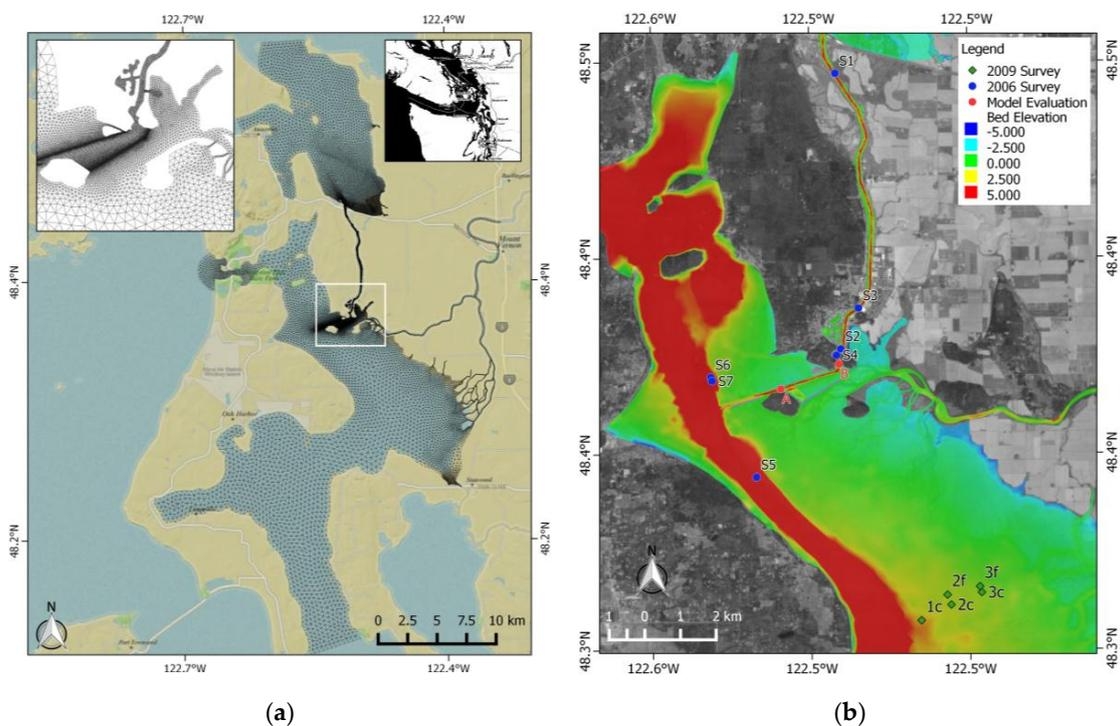
**Figure 2.** (a) The Skagit River estuary model grid with expanded domain covering Padilla Bay to the north and Saratoga Passage to the South with the Swinomish Channel connecting the two basins; (b) the locations of May 2006 (blue circles), WHOI study mooring stations during June of 2009 [13] (green diamonds), and for scenario evaluation (red circles).
