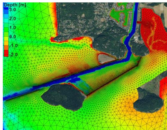
**Figure 8.** Close-up of the model grid and bathymetry used in baseline (or existing conditions) simulation. Note—color contours indicate depths (negative elevations) relative to NAVD88 datum.
