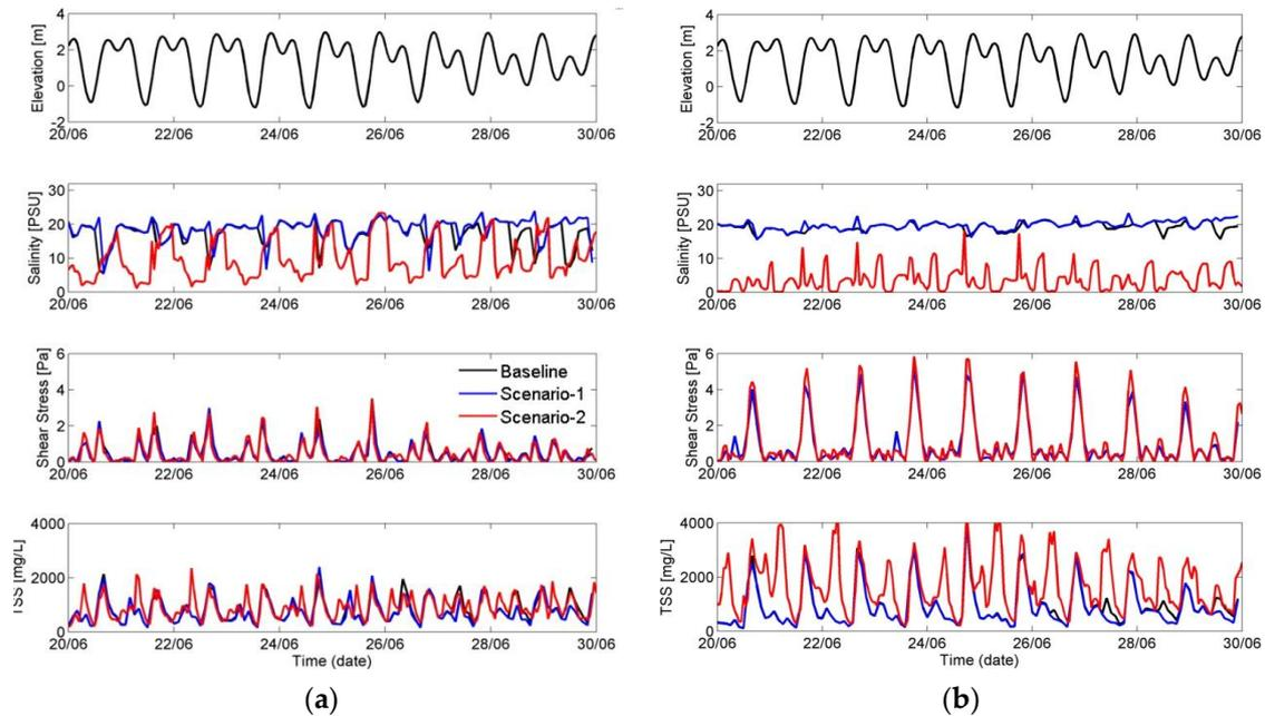
**Figure 17.** Comparison of time series of salinity, bed shear stress and TSS at (a) station A and (b) station B (Figure 2b) for baseline, Jetty Repair Scenario, SCN-1, and McGlinn Causeway restoration, SCN-2.
