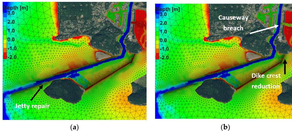
**Figure 9.** Modified model configuration used for (a) SCN-1 South Jetty Repair and (b) SCN-2, McGlinn Causeway Restoration. Note—color contours indicate depths (negative elevations) relative to NAVD88 datum.
