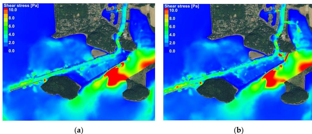
**Figure 14.** Time averaged bottom shear stress distribution (20 days) for (a) baseline conditions and (b) McGlinn Causeway restoration, SCN-2.
