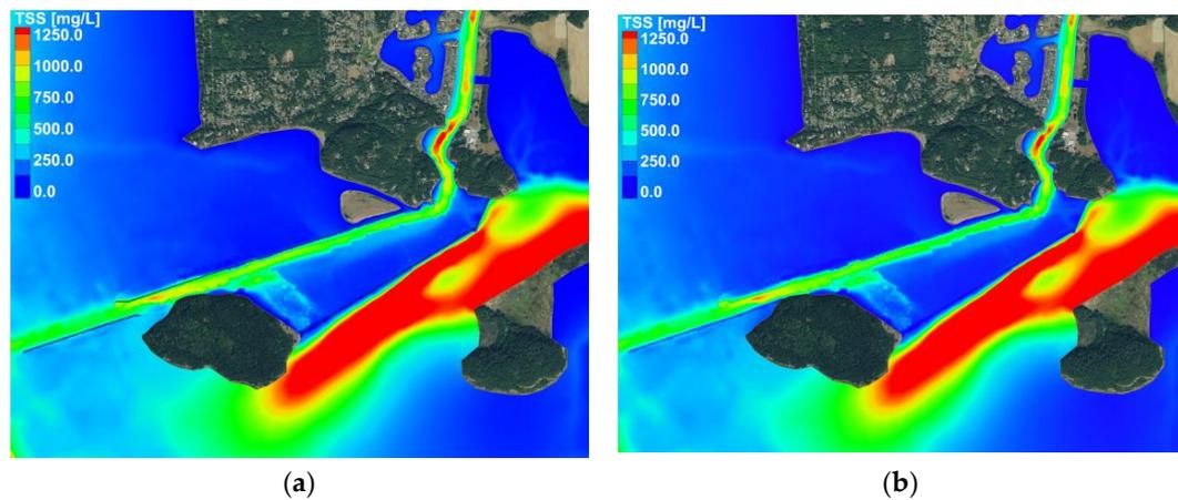
**Figure 12.** Time averaged total suspended sediment (TSS) distribution (20 days) for (a) baseline conditions and (b) Jetty Repair Scenario, SCN-1.
