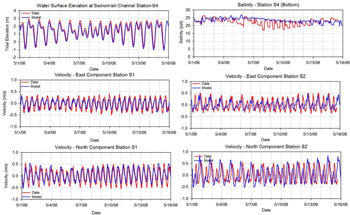
**Figure 3.** Comparison of observed tide, salinity, and currents in the Swinomish Channel (Figure 2b) shown as example at stations S1, S2, and S4 during May of 2006 as part of hydrodynamic model setup and calibration.
