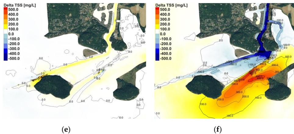
**Figure 16.** Time averaged horizontal distribution difference between baseline conditions and SCN-1 for (a) salinity (c) shear stress and (e) TSS; time averaged horizontal distribution difference between baseline conditions and SCN-2 for (b) salinity (d) shear stress and (f) TSS. The positive sign of the color bar means that the baseline concentrations are higher than the selected scenario.
