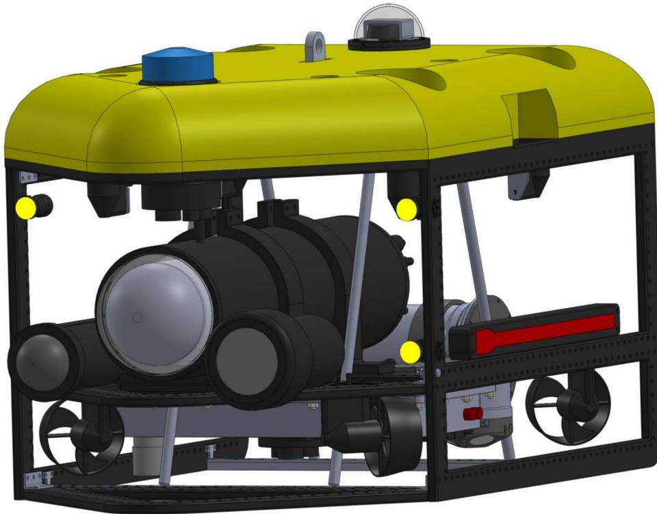
**Figure 1.** Inspection-class remotely operated vehicle (I-ROV), developed at the Centre for Robotics & Intelligent Systems (CRIS) researchers, University of Limerick (UL).
