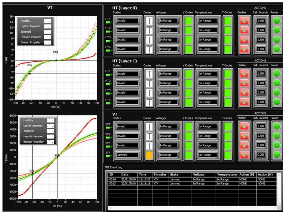
Figure 18. Thruster FDI result for thruster state = "Jammed".
