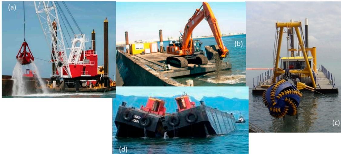
**Figure 6.** Examples of marine construction equipment: (a) A clamshell bucket grab; (b) a barge-mounted backhoe; (c) a cutter suction head and support vessel; and (d) a split hull barge used for disposal at sea.
