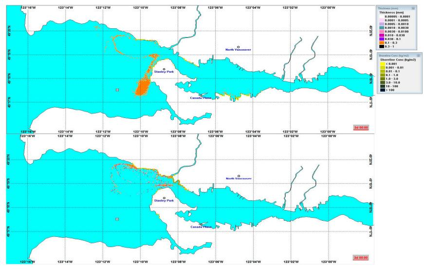
Figure S2. Example of oil trajectories for spilled oil forced without wind (top) or with wind (bottom).
