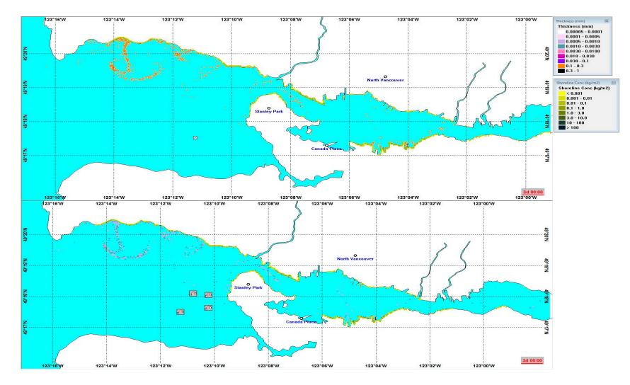
**Figure S4.** Example of oil trajectories for oil spill without (top) or taken (bottom) recovery actions. **Table S7.** Water surface contaminant comparison. The simulated results were compared with observation data.
