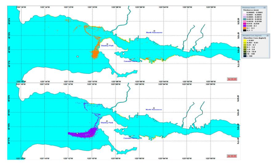
Figure S3. Example of oil trajectories for oil discharge instantly (top) or continuously (bottom).
