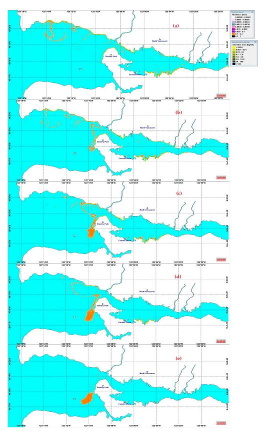
**Figure S1.** Example of oil trajectories for oil spill with different oil start-releasing time. Figures from top to bottom are oil start release oil at (a) 12:00, (b) 13:00, (c) 14:00, (d) 15:00, and (e) 16:00.
