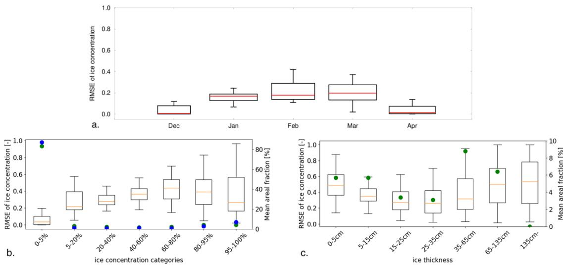
**Figure 8.** Ranges of spatial concentration RMSE as functions of month (a), ice concentration (b) and ice thickness (c) for Lake Michigan from the LMHOFS 2015–2017 simulation results. See the caption of Figure 5 for the explanation of the box, whiskers, and solid circles. For (c), open water cells are excluded.
