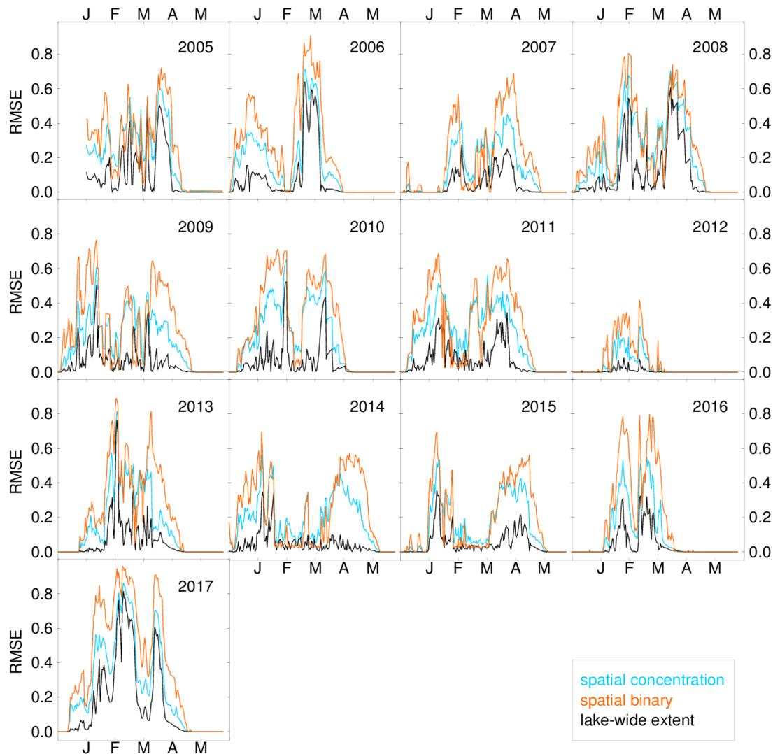
**Figure 4.** Time series of ice simulation errors between the Lake Erie model and the NIC based on the three methods: Pixel-to-pixel RMSE based on ice concentration (**cyan**), pixel-to-pixel RMSE based on binary ice cover (**orange**), and lake-wide absolute error (**black**). Please note that lake-wide absolute error shows only the magnitude of error (i.e., does not show the sign of model bias).
