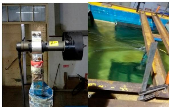
Figure 4. Testing of thrusters (left: fixing method; right: testing with current).
