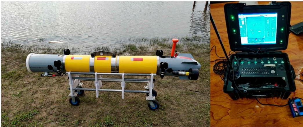
Figure 2. Plateau data-gathering AUV system (left: developed AUV; right: ground station).
