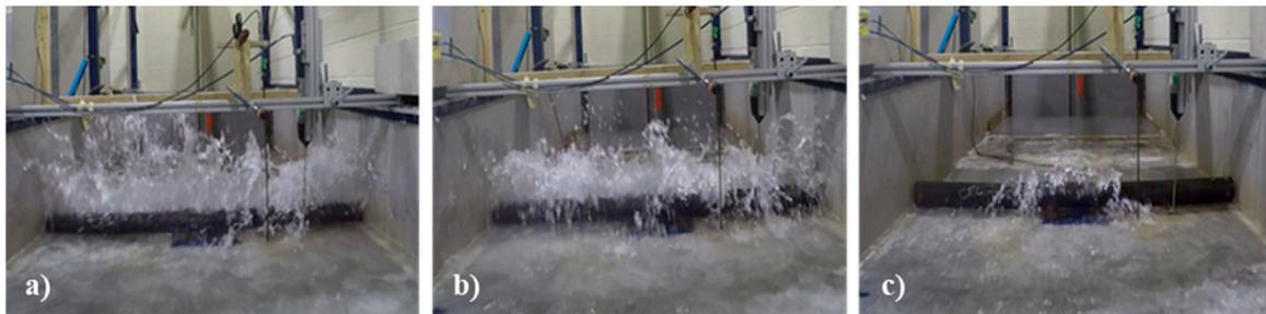
**Figure 7.** Bore impact on the pipe for three impundment depths: (a)  $h = 50$  cm, (b)  $h = 40$  cm, and (c)  $h = 30$  cm.
