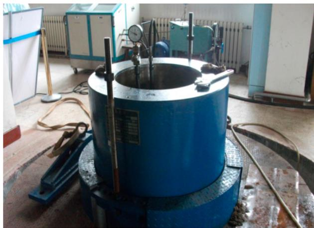
**Figure 12.** The pressure test chamber.
