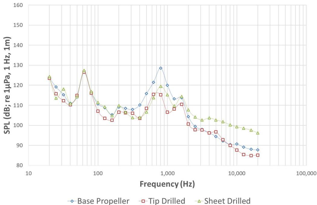
**Figure 5.** Comparative sound pressure levels of three model propellers tested for  $J = 0.50$  and cavitation condition. Reproduced from [13] with permission from Newcastle University.
