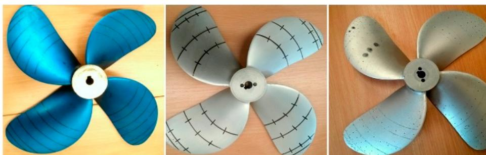
**Figure 2.** From left to right: “Base” propeller; “Tip” (region) modified propeller; and mid and tip (region) modified, “Sheet” propeller. Reproduced from [13] with permission from Newcastle University.
