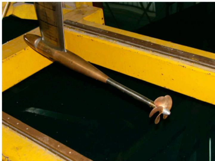
Figure 10. CTO Towing tank open water test set-up.
