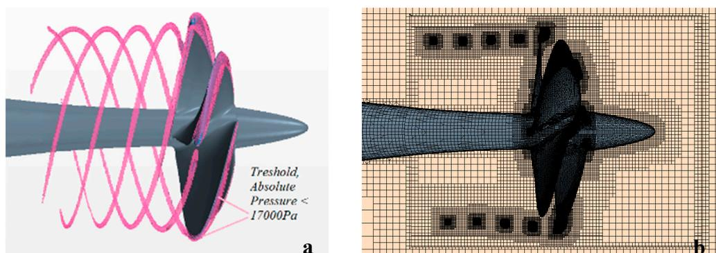
**Figure 21.** Tip vortex cavitation refinement (MARCS); (a) Left; Treshold Region, (b) Right; Generated Mesh.
