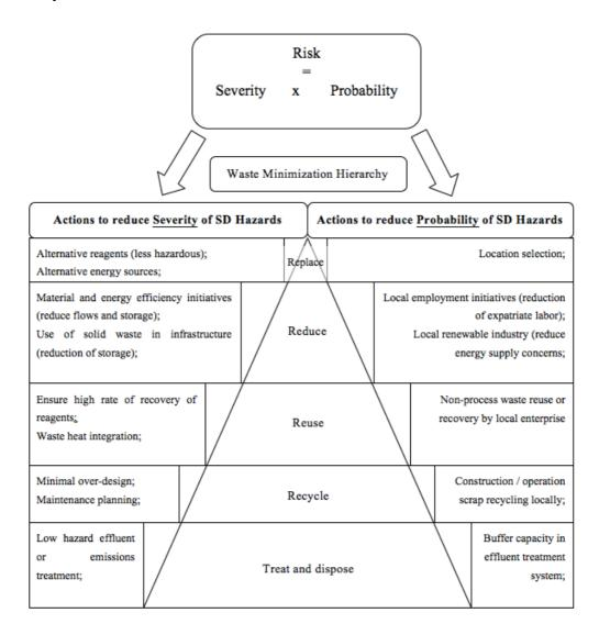
**Figure 1.** Waste minimization hierarchy and its relationship to reducing the severity and probability of hazards.
