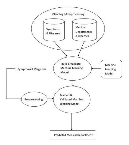
Figure 3. Block Diagram of the System Implemented.
