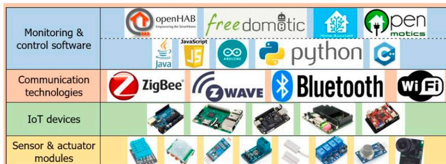
**Figure 2.** Information and Communication Technology (ICT) components for data acquisition in Smart Energy-Efficient Buildings (SEEB).
