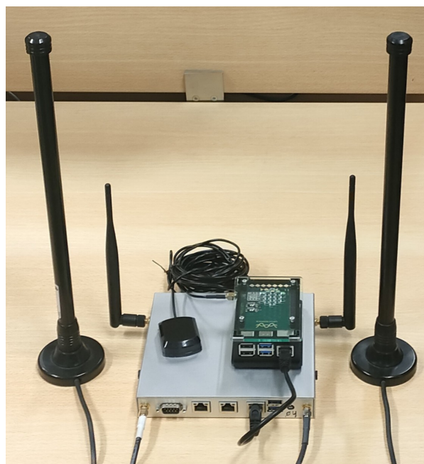
Figure 8. An RSU used for performance analysis of the proposed implemented system. It is connected via Ethernet to a Raspberry Pi which functions as a timeserver. The pair of larger antennas are used for ITS-G5 communications, while the pair of smaller antennas are used for LTE communications.
