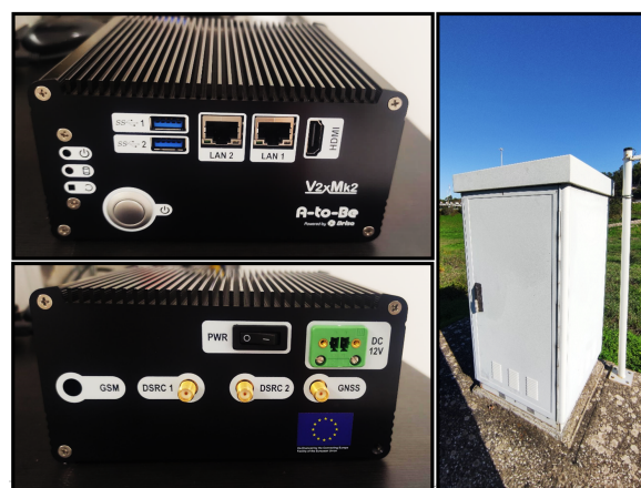
Figure 2. A deployed RSU. It is pictured: the front of the RSU ( top left ) with frontal power switch and USB, Ethernet and HDMI ports; the back of the RSU ( bottom left ) with back power switch, power socket and GSM/LTE, DSRC (ITS-G5) and GNSS antenna connectors; and the housing of the RSU adjacent to a motorway ( right ).
