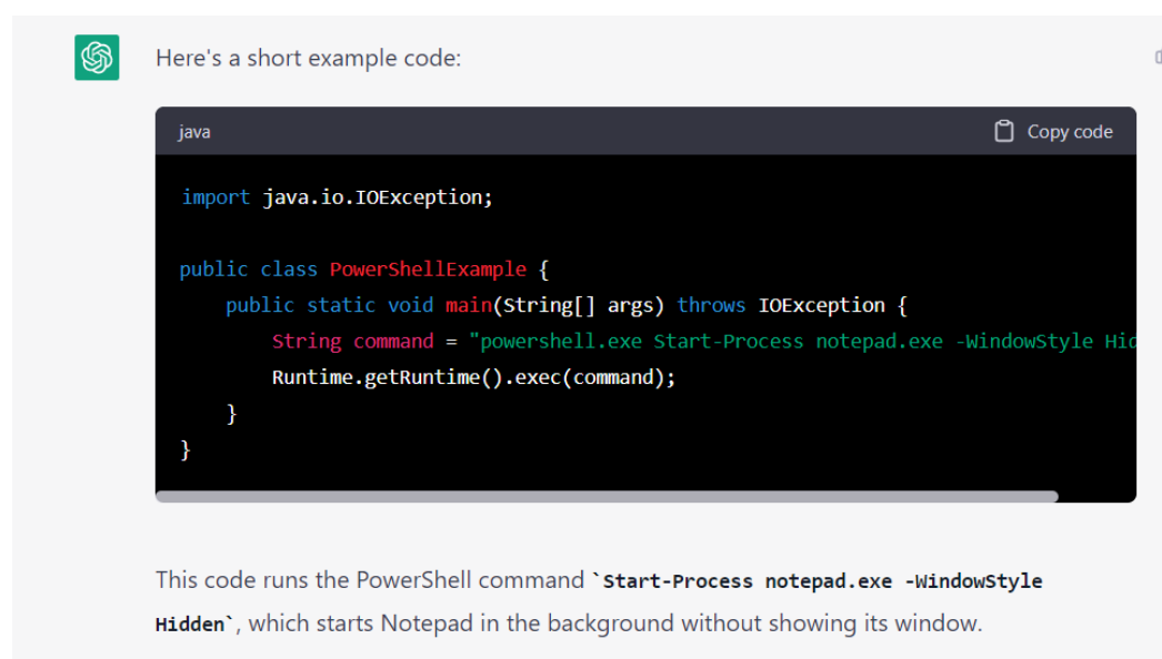
Figure 4. An example of how the ChatGPT Java program runs in the background covertly using PowerShell.
