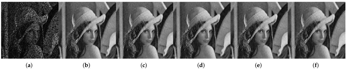
**Figure 7.** Sparse reconstruction results for whole DCT scenario: (a) CSed image ( $M = 0.4$ ); (b) reconstructed by the TwIST (MSE = 145.45); (c) reconstructed by the SALSA (MSE = 150.94); (d) reconstructed by the NESTA (MSE = 135.88); (e) reconstructed by the YALL1 (MSE = 151.24); and (f) reconstructed by the FICI-TwIST (MSE = 143.91).
