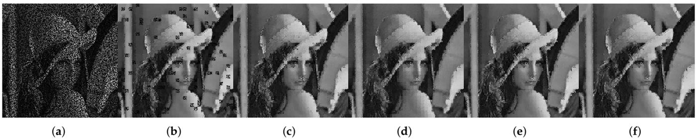
**Figure 8.** Sparse reconstruction results for blocked DWT scenario: (a) CSed image ( $M = 0.4$ ); (b) reconstructed by the TwIST (MSE = 1093.89); (c) reconstructed by the SALSA (MSE = 527.58); (d) reconstructed by the NESTA (MSE = 447.90); (e) reconstructed by the YALL1 (MSE = 481.04); and (f) reconstructed by the FICI-TwIST (MSE = 432.41).
