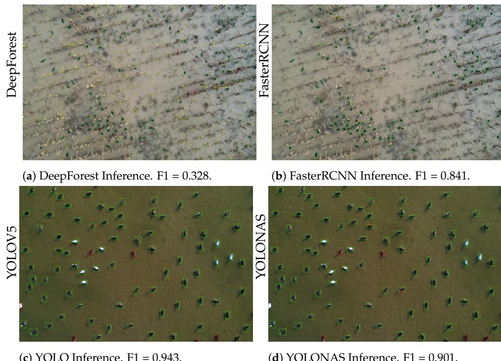
**Figure 3.** Detection results of the DeepForest Bird Detector: (a) Faster R-CNN. (b) YOLOv5. (c) YOLONAS. (d) An image of a flooded corn field. In each image, green boxes denote True Positive (TP) predictions, yellow boxes denote False Positive (FP) predictions, and red boxes denote False Negative (FN) predictions.
