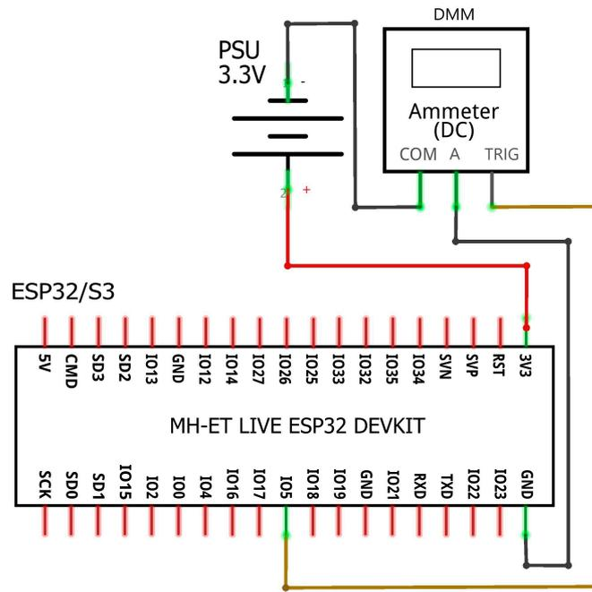
Figure 1. Block diagram of device's connections.
