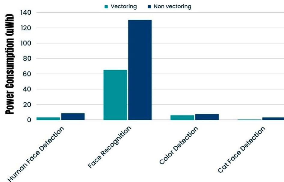
**Figure 5.** Power consumption with and without SIMD/vectoring operation extensions.
