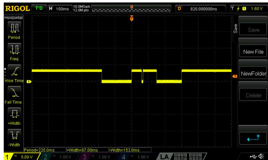
Figure 3. Captured trigger signal of color detection model.
