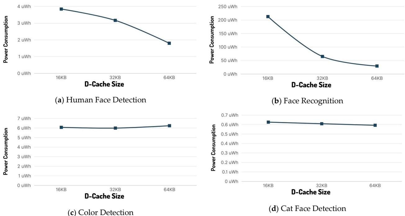
**Figure 4.** Power consumption vs. cache size.
