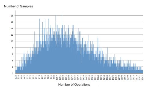
In Figure 6, we can say that the distribution found is a log-normal distribution, because we had  $AD=0.153 < AD_{\rm critical}=1.035$ . We show the tests of compliance for this data with the gamma distribution with 3 parameters (Figure 6a), and with the log-normal distribution with 3 parameters (Figure 6b). The latter displays a better compliance with the log-normal distribution.
