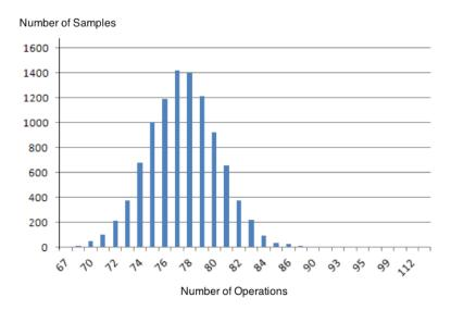
**Low-medium:**  $\frac{m}{n} = 3$  As the ratio  $\frac{m}{n}$  increases, the tail of the distribution begins to extend to the right and also increases the frequency of events. The distance between points decreases, approaching a continuous distribution. Figure 3 is an example for n = 50 and m = 150.
