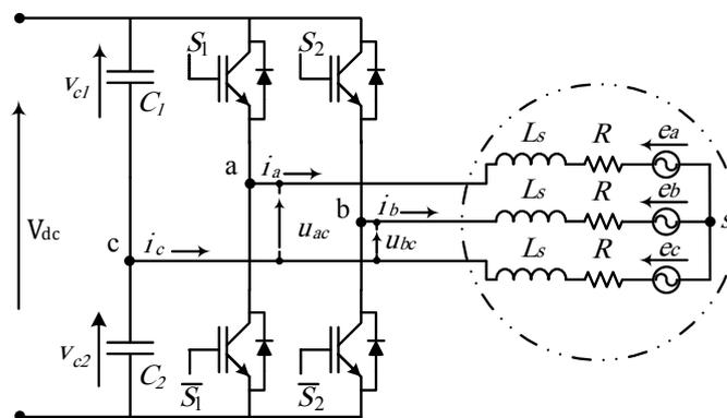
Figure 1. Power circuit of the four-switch three-phase inverter.
