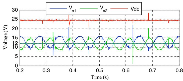
**Figure 10.** Capacitor voltages' fluctuation at 200 rpm when the proposed control scheme is applied.
