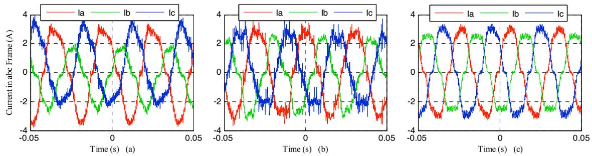
**Figure 8.** Experimental waveforms of the three-phase motor current  $I_a$ ,  $I_b$  and  $I_c$ , when the load is applied at 500 rpm. (a) Motor phase current with the standard control scheme; (b) Motor phase current with the proposed control scheme; (c) Motor phase current when the six-switch three-phase inverter is used.
