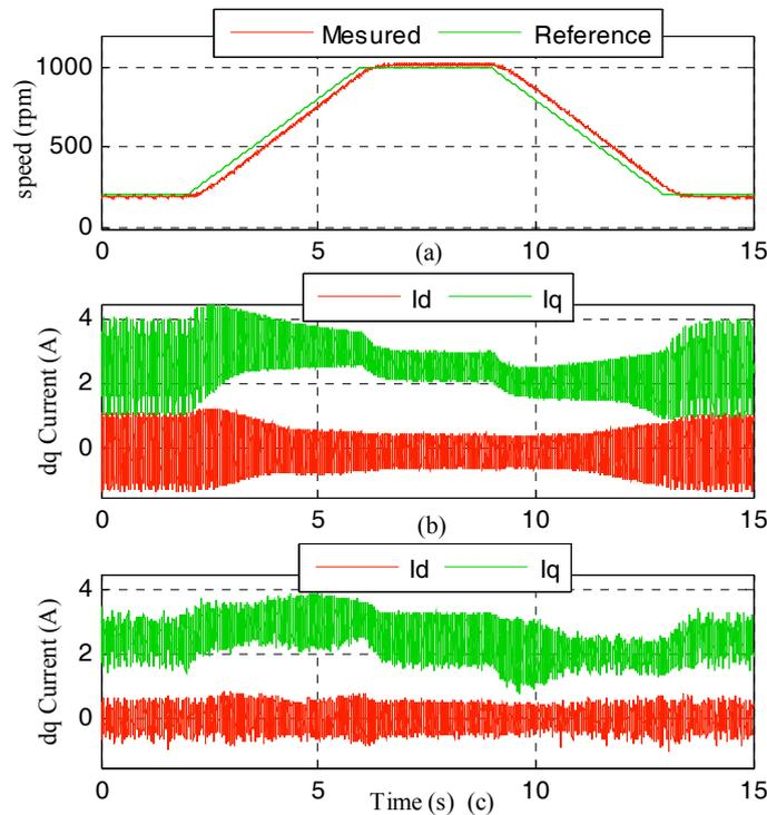
**Figure 11.** Experimental result of speed profile following. (a) Reference and measured speed; (b) motor currents in the d-q frame without compensation scheme; (c) motor currents in the d-q frame with the proposed scheme.
