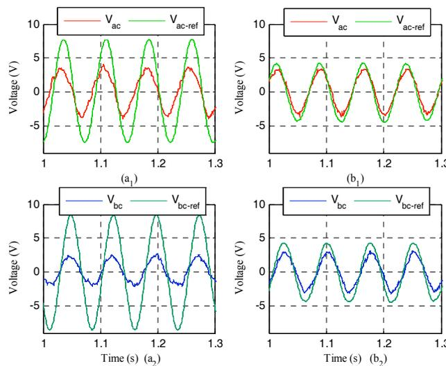
**Figure 7.** Experimental results at 200 rpm of controlled 4S3P output voltages compared to their references: (a1,a2) are without compensation; (b1,b2) are with the proposed scheme.
