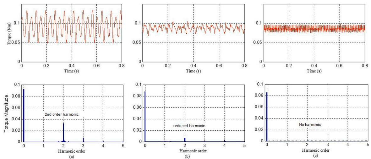
**Figure 9.** Experimental waveforms of the motor torque and their frequency analyses under a load at 200 rpm. (a) With the standard control scheme; (b) With the proposed control scheme; (c) When the six-switch three-phase inverter is used.
