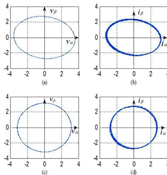
**Figure 5.** Simulation of voltage and current trajectories in the  $\alpha$ - $\beta$  reference frame at 200 rpm; (a,b) are the voltage and current wave form without voltage regulation; (c,d) are the voltage and current wave form with the proposed voltage control scheme.
