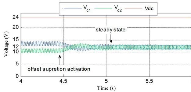
**Figure 6.** Simulation result of the capacitors' voltage  $V_{c1}$ ,  $V_{c2}$  and  $V_{dc}$  behaviors at the activation of the voltage offset suppression, at 800 rpm.
