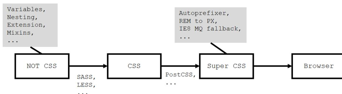
**Figure 1.** The CSS workflow with the two CSS processor types.
