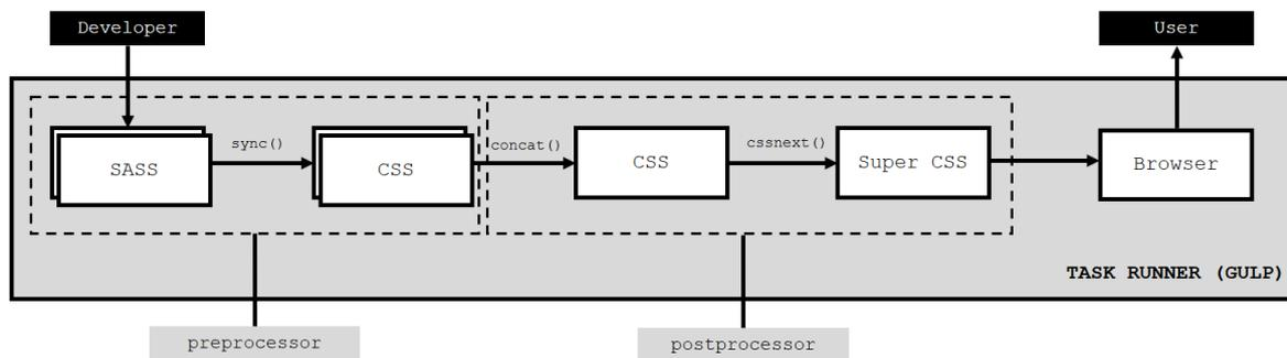
Figure 4. The CSS workflow with the two CSS processor types.
