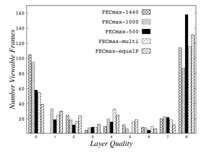
**Figure A4.** Example of the number of viewable layers for SVC-SC, for each of the  $FEC_{max}Packet_{thres}$ , at a packet loss rate of 10%.
