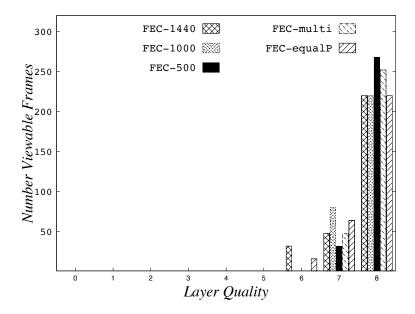
**Figure A20.** Example of the number of viewable layers for SVC-SC, for each of the *FECPacket*<sub>thres</sub>, at a packet loss rate of 10% and a GOP of 16. This image illustrates an increase in the *FEC* for C1 and C2 based on the worst case scenario, as shown in Table A2.
