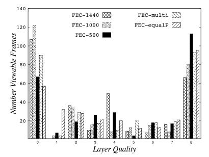
**Figure A3.** Example of the number of viewable layers for SVC-SC, for each of the *FECPacket*<sub>thres</sub>, at a packet loss rate of 10%.
