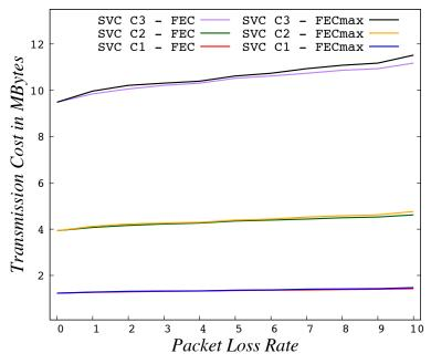
**Figure A2.** Transmission cost for the SVC-SC classes C1, C2 and C3 for both FEC and *FEC*<sub>max</sub> with packet loss rates from 0 to 10%.
