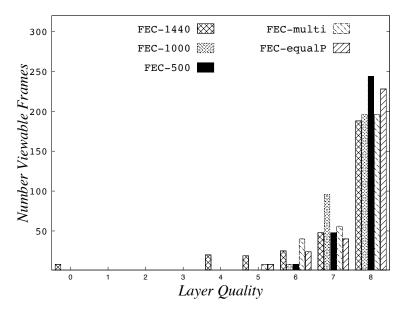
**Figure A14.** Example of the number of viewable layers for SVC-SC, for each of the  $FEC_{max}Packet_{thres}$ , at a packet loss rate of 10% and a GOP of 8. This image illustrates an increase in the  $FEC_{max}$  for C1 and C2 based on the worst case scenario, as shown in Table A2.
