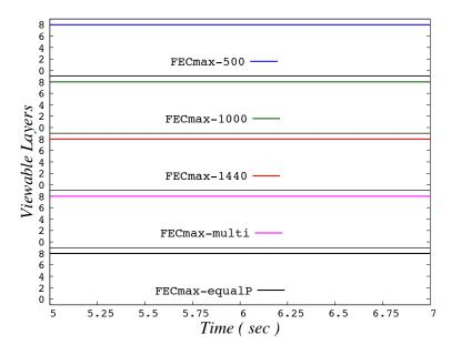
**Figure A25.** A two-second example of variation in viewable quality for all  $FEC_{max}$  models, at a packet loss rate of 10% and a GOP of 32. This illustrates an increase in the  $FEC_{max}$  for C1 and C2 based on the worst case scenario, as shown in Table A2.
