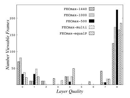
**Figure A10.** Example of the number of viewable layers for SVC-SC, for each of the  $FEC_{max}Packet_{thres}$ , at a packet loss rate of 10% and a GOP of 8.
