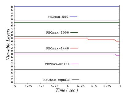
**Figure A22.** A two-second example of variation in viewable quality for all  $FEC_{max}$  models, at a packet loss rate of 10% and a GOP of 16. This illustrates an increase in the  $FEC_{max}$  for C1 and C2 based on the worst case scenario, as shown in Table A2.
