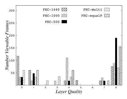
**Figure A16.** Example of the number of viewable layers for SVC-SC, for each of the *FECPacket*<sub>thres</sub>, at a packet loss rate of 10% and a GOP of 16.
