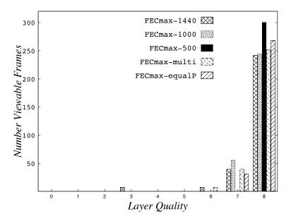
**Figure A13.** Example of the number of viewable layers for SVC-SC, for each of the *FECPacket*<sub>thres</sub>, at a packet loss rate of 10% and a GOP of 8. This image illustrates an increase in the *FEC* for C1 and C2 based on the worst case scenario, as shown in Table A2.
