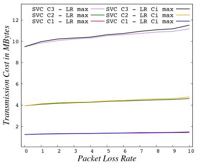
**Figure A1.** Transmission cost for the SVC-SC classes C1, C2 and C3 for both  $LR_{max}$  and  $LR_{C_i}^{max}$  with packet loss rates from 0 to 10%.
