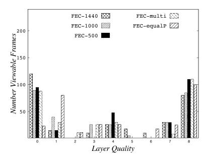
**Figure A9.** Example of the number of viewable layers for SVC-SC, for each of the *FECPacket*<sub>thres</sub>, at a packet loss rate of 10% and a GOP of 8.
