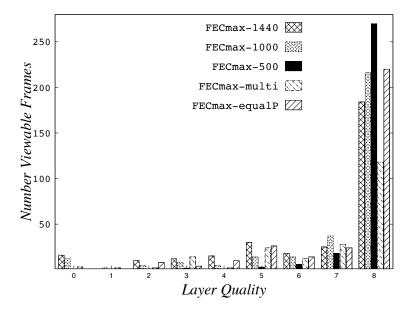
**Figure A8.** Example of the number of viewable layers for SVC-SC, for each of the  $FEC_{max}Packet_{thres}$ , at a packet loss rate of 10%. This image illustrates an increase in the  $FEC_{max}$  for C1 and C2 based on the worst case scenario, as shown in Table A2.
