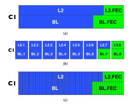
**Figure 8.** Examples of two layers allocated to class one ( $C_1$ ) for (**a**) SVC plus FEC and (**b**) description-based models plus FEC; (**b**) illustrates the section structure of MDC utilised by IRP, while (**c**) illustrates an example of the IRP packetisation of the SVC class in (**a**).
