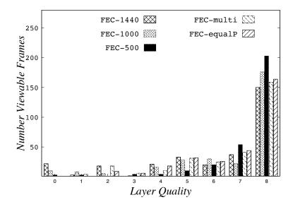
**Figure A7.** Example of the number of viewable layers for SVC-SC, for each of the *FECPacket*<sub>thres</sub>, at a packet loss rate of 10%. This image illustrates an increase in the *FEC* for C1 and C2 based on the worst case scenario, as shown in Table A2.
