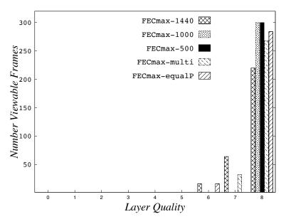
**Figure A21.** Example of the number of viewable layers for SVC-SC, for each of the  $FEC_{max}Packet_{thres}$ , at a packet loss rate of 10% and a GOP of 16. This image illustrates an increase in the  $FEC_{max}$  for C1 and C2 based on the worst case scenario, as shown in Table A2.
