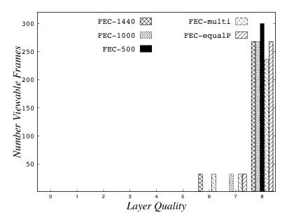
**Figure A23.** Example of the number of viewable layers for SVC-SC, for each of the *FECPacket*<sub>thres</sub>, at a packet loss rate of 10% and a GOP of 32. This image illustrates an increase in the *FEC* for C1 and C2 based on the worst case scenario, as shown in Table A2.
