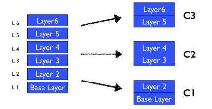
Figure 4. Example of a six-layer SVC stream grouped as three hierarchical classes.
