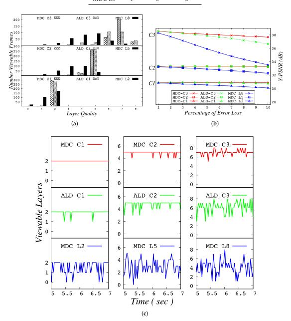
**Figure 16.** Performance evaluation of considered schemes using IRP for SCs. (**a**) video quality for different schemes at 10% loss; (**b**) average Y-PSNR values for different schemes with 95% confidence interval results; (**c**) 2 s sample of viewable quality transitions.
