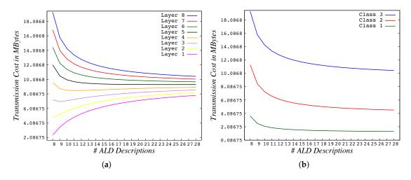
**Figure 14.** Transmission cost of the crew media clip for (**a**) each layer; and (**b**) each streaming class, as the STF value and associated number of ALD descriptions increase.
