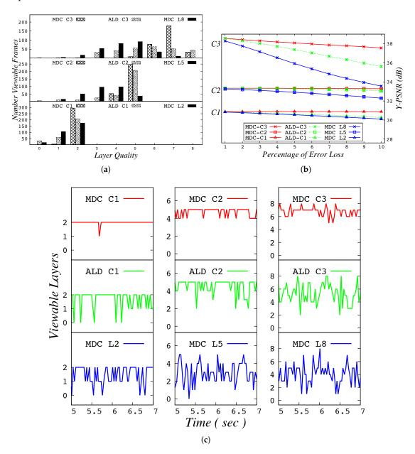
**Figure 15.** Performance evaluation of considered schemes using ROP for SCs. (**a**) video quality for different schemes at 10% loss; (**b**) average Y-PSNR values for different schemes with 95% confidence interval results; (**c**) 2 s sample of viewable quality transitions for MDC (layers L2, L5 and L8) and for each of the classes of ALD-SC and MDC-SC (maximum quality per class equating to layers 2, 5 and 8).
