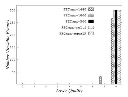
**Figure A24.** Example of the number of viewable layers for SVC-SC, for each of the  $FEC_{max}Packet_{thres}$ , at a packet loss rate of 10% and a GOP of 32. This image illustrates an increase in the  $FEC_{max}$  for C1 and C2 based on the worst case scenario, as shown in Table A2.
