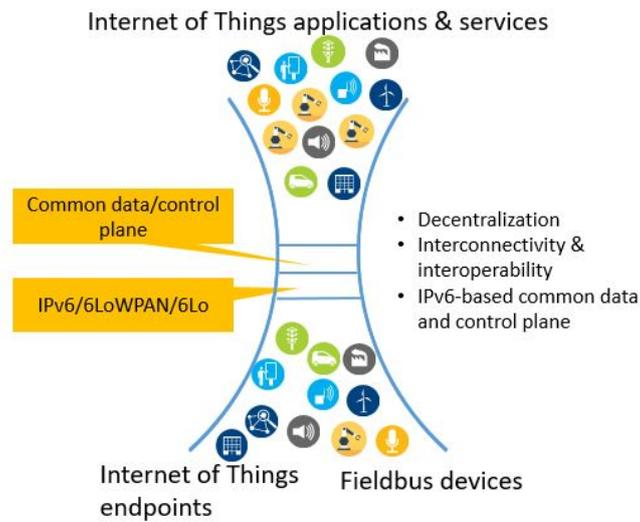
**Figure 1.** Convergence towards a common IPv6-based data and control plane connecting Internet of Things (IoT) endpoints and fieldbus devices with decentralised applications and services.
