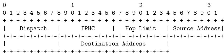
Figure 6. Compressed IPv6 header.
