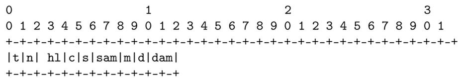
Figure 15. RoHC IPv6 header frame format.
