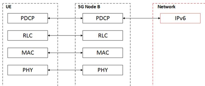
**Figure 4.** 5G architecture stack outline comprising a physical layer (PHY), medium access control (MAC) layer, radio link control (RLC) layer and a packet data convergence protocol (PDCP) layer. IPv6 packets would flow between the networking layer and the Packet Data Convergence Protocol layer, which we depict in red in this diagram.
