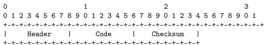
Figure 16. Ultra-compressed IPv6 ICMPv6 message for LoRaWAN.
