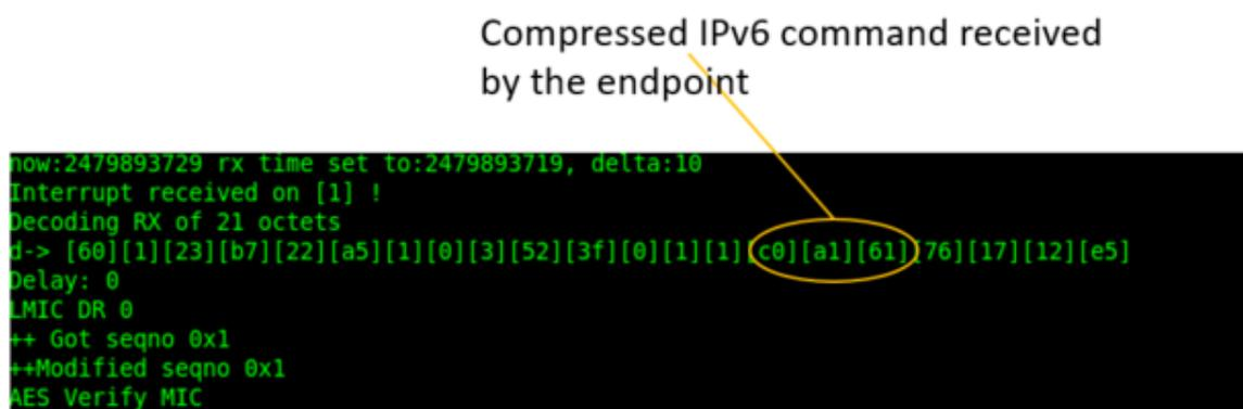
**Figure 22.** Received downstream bytes reported by a LoRaWAN test endpoint.
