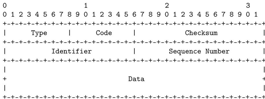
Figure 14. ICMPv6 echo request packet format.
