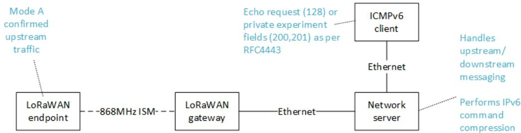
**Figure 18.** Experimental configuration—we used the 868 MHz industrial, scientific, and medical (ISM) radio band with LoRaWAN Mode A and confirmed upstream traffic.
