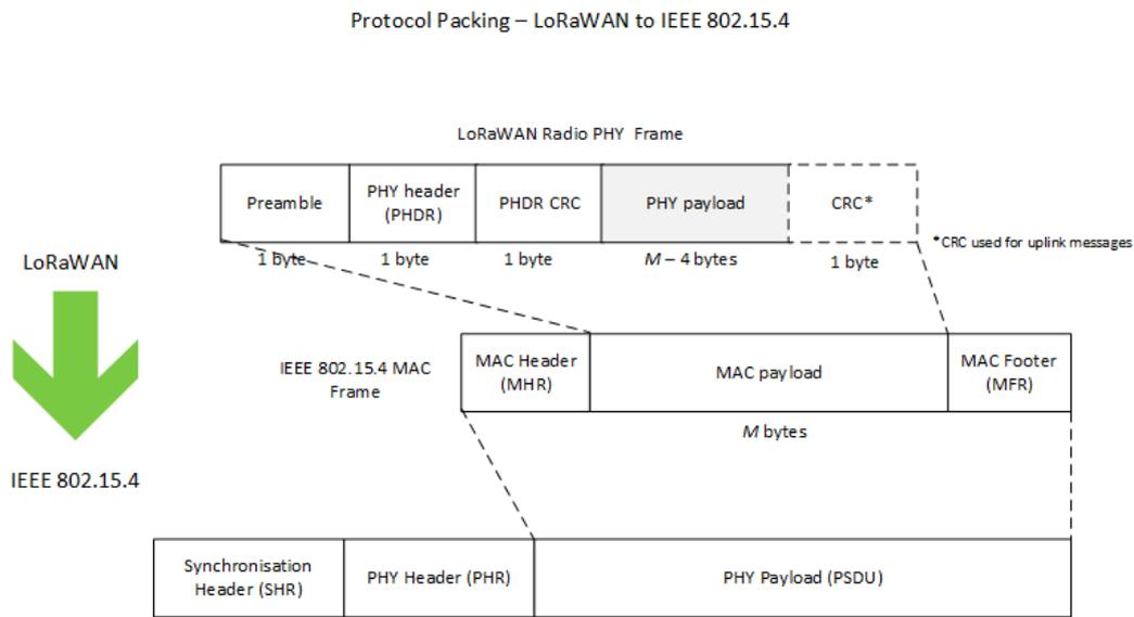
**Figure 7.** Packing LoRaWAN frames inside an IEEE 802.15.4 MAC frame.
