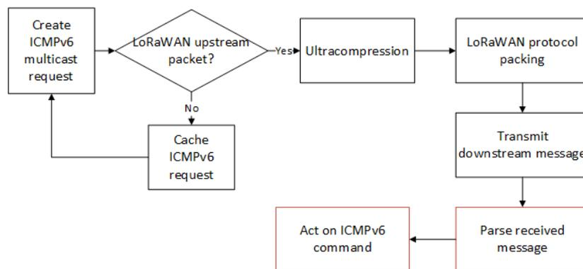
Figure 17. Main processes involved for the downstream handling of ICMPv6 commands and LoRaWAN messaging.
