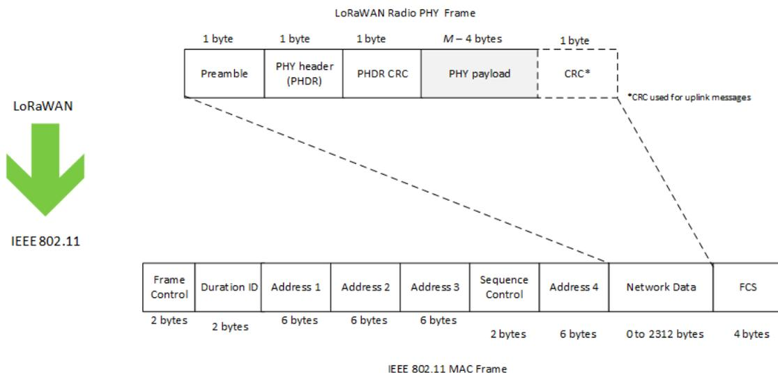
**Figure 8.** Packing LoRaWAN frames inside an IEEE 802.11 MAC frame.
