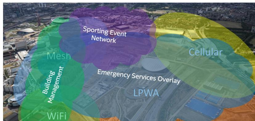
**Figure 2.** Complex multitopology heterogeneous WiFi, low power wide area (LPWA), mesh, and cellular networks with a common data and control plane supporting multiple different applications and services.
