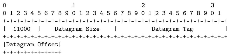
Figure 10. Second and subsequent fragmentation header.
