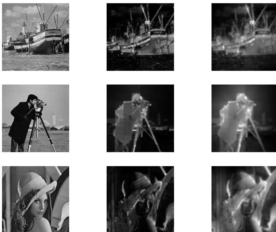
Figure 2. The saliency estimation result of the proposal method in comparison with the MSNR method. From left to right: the original image, the saliency map generated by MSNR method and the saliency map generated by proposal method.
