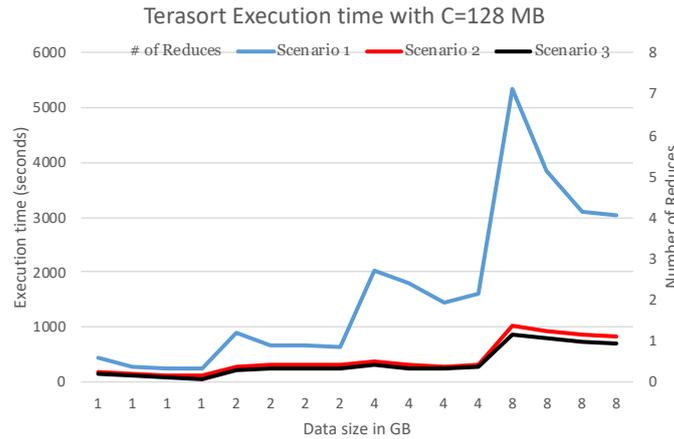
**Figure 7.** Comparison of Terasort execution times for Scenarios 1, 2, and 3. The data sizes are 1 GB, 2 GB, 4 GB, and 8 GB, with number of reduce tasks = 1, 2, 4, and 8. Chunk size C = 128 MB.
