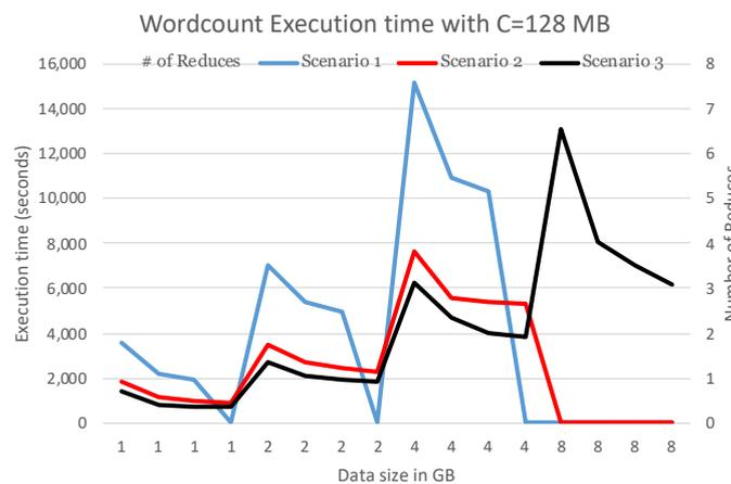
**Figure 8.** Comparison of WordCount execution times for Scenarios 1, 2 and 3. The data sizes are 1 GB, 2 GB, 4 GB, and 8 GB with number of reduce tasks = 1, 2, 4, and 8. Chunk size C = 128 MB.
