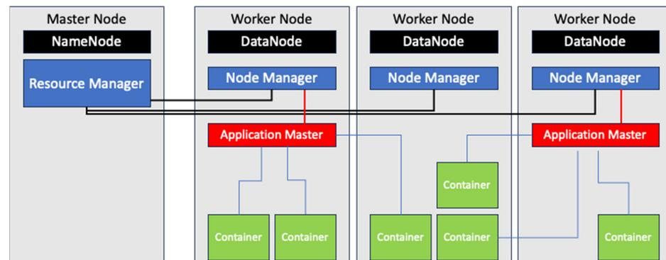
**Figure 1.** Hadoop YARN architecture and service flow.
