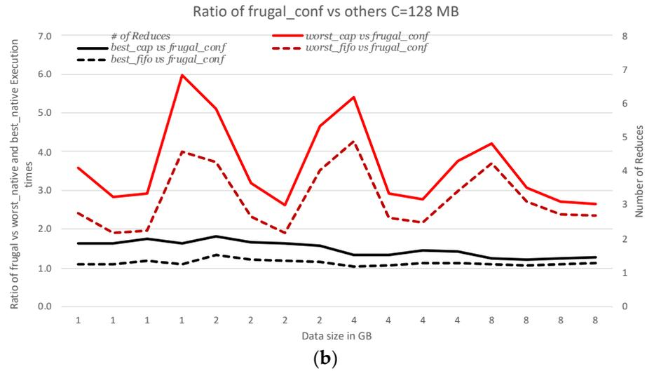
**Figure 6.** Comparison of Terasort execution time ratios of *frugal\_conf* vs. *best\_cap*, *worst\_cap*, *best\_fifo*, and *worst\_fifo*. The data sizes are 1 GB, 2 GB, 4 GB, and 8 GB with number of reduce tasks = 1, 2, 4, and 8. (a) Chunk size C = 64 MB. (b) Chunk size C = 128 MB.
