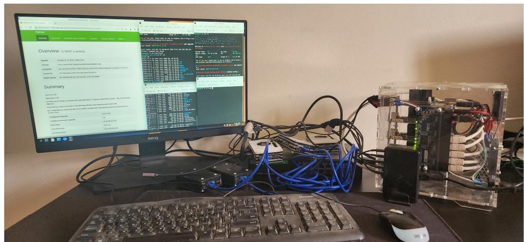
Figure 4. Heterogeneous Hadoop cluster built with frugal SBC devices, including RPi5, RPi3, Odroid Xu4, and RockPro64. One of the RPi5 serves as the master while the rest of the SBCs run the worker nodes. All the SBCs are connected to a Gigabit Ethernet switch.
