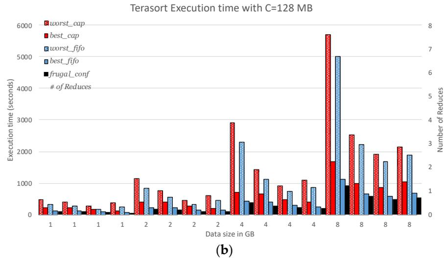
**Figure 5.** Execution times of various Terasort jobs with varying dataset sizes, 1 GB, 2 GB, 4 GB, and 8 GB, and number of reduce tasks = 1, 2, 4, and 8. (a) Chunk size C = 64 MB. (b) Chunk size C = 128 MB.
