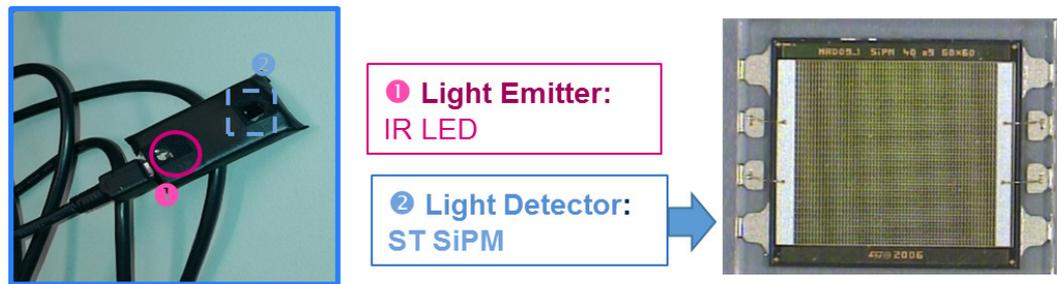
Figure 2. Silicon Photomultiplier (SiPM) detector filter and PPG probe.
