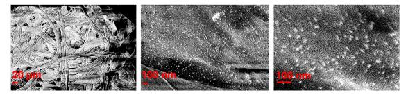
**Figure S5.** SEM images at different magnifications of the plasmonic paper exposed to solution containing 50 mM ferricyanide and 10  $\mu$ g mL<sup>-1</sup>BSA (20 min).
