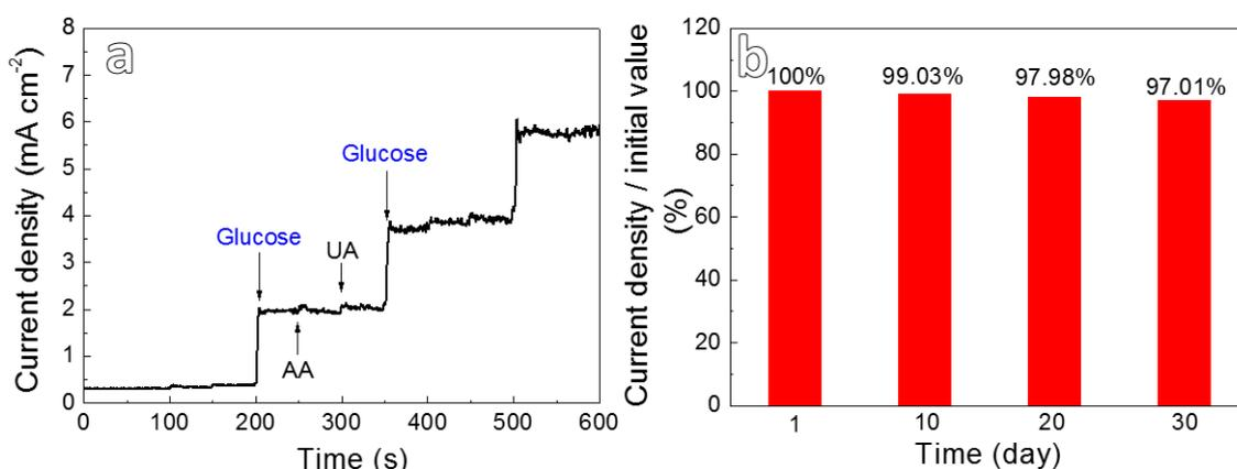
**Figure 6.** (a) Anti-interference ability measurement of  $\text{Cu}_x\text{O}/\text{Ag}_2\text{O}$ -10 at an applied potential of 0.5 V; (b) the stability of the  $\text{Cu}_x\text{O}/\text{Ag}_2\text{O}$ -10 electrode over a period of 30 days.
