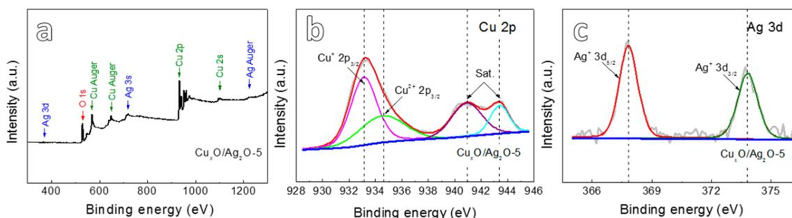
**Figure 3.** (a) XPS spectrum of the  $\text{Cu}_x\text{O}/\text{Ag}_2\text{O}-5$ ; (b) Cu 2p XPS spectrum of  $\text{Cu}_x\text{O}/\text{Ag}_2\text{O}-5$ ; (c) Ag 3d XPS spectrum of  $\text{Cu}_x\text{O}/\text{Ag}_2\text{O}-5$ .
