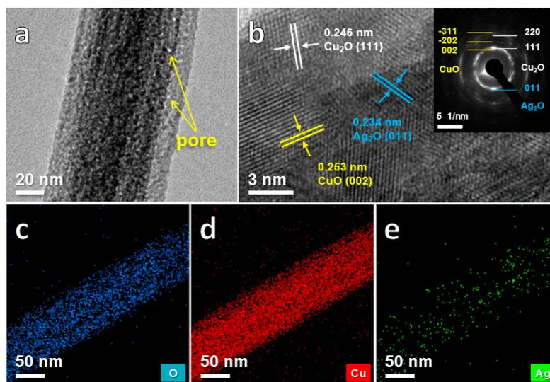
**Figure 4.** TEM images of the  $\text{Cu}_x\text{O}/\text{Ag}_2\text{O}$ -5 nanowires (a) high magnification image; (b) HRTEM image with the SAED pattern; the EDS elemental mapping images of (c) O; (d) Cu; (e) Ag.
