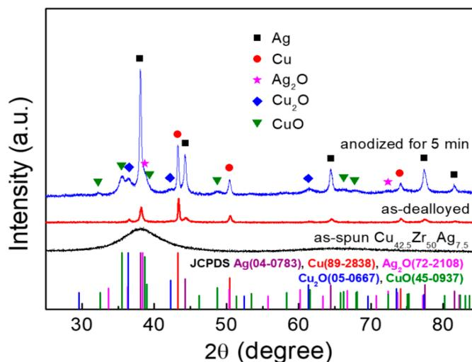
**Figure 2.** XRD patterns of the as-spun, as-dealloyed and as-prepared sample after anodizing for 5 min followed by calcination.
