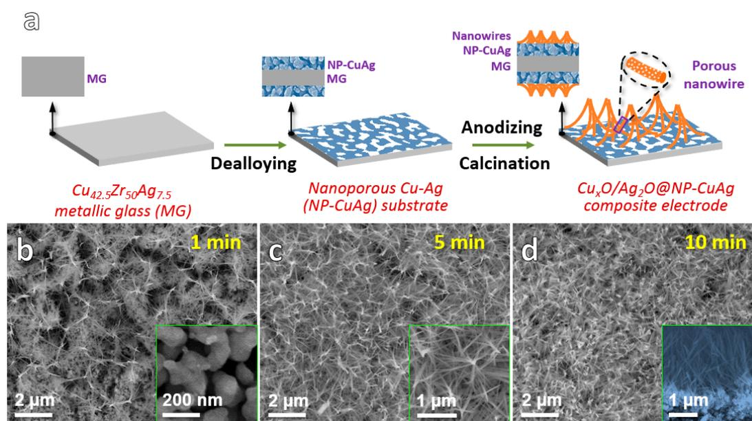
**Figure 1.** (a) Schematic illustration showing the synthesis process of  $\text{Cu}_x\text{O}/\text{Ag}_2\text{O}@NP\text{-CuAg}$  composite; SEM images of  $\text{Cu}_x\text{O}/\text{Ag}_2\text{O}@NP\text{-CuAg}$  anodized for different time followed by calcination (b) 1 min with the inset of NP-CuAg substrate; (c) 5 min and the magnification image; (d) 10 min with the sectional image.
