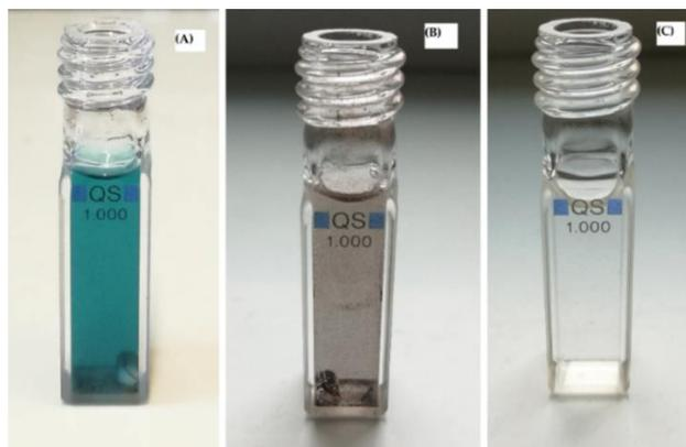
**Figure 11.** Visual representation of MB degradation in photo-Fenton process in the photo-reactor (cuvette). (A) Mixture of MB + NP-3 before photocatalysis, (B) MB + NP-3 after photocatalysis, and (C) clear solution obtained after separation (centrifugation) of solid catalyst from (B).
