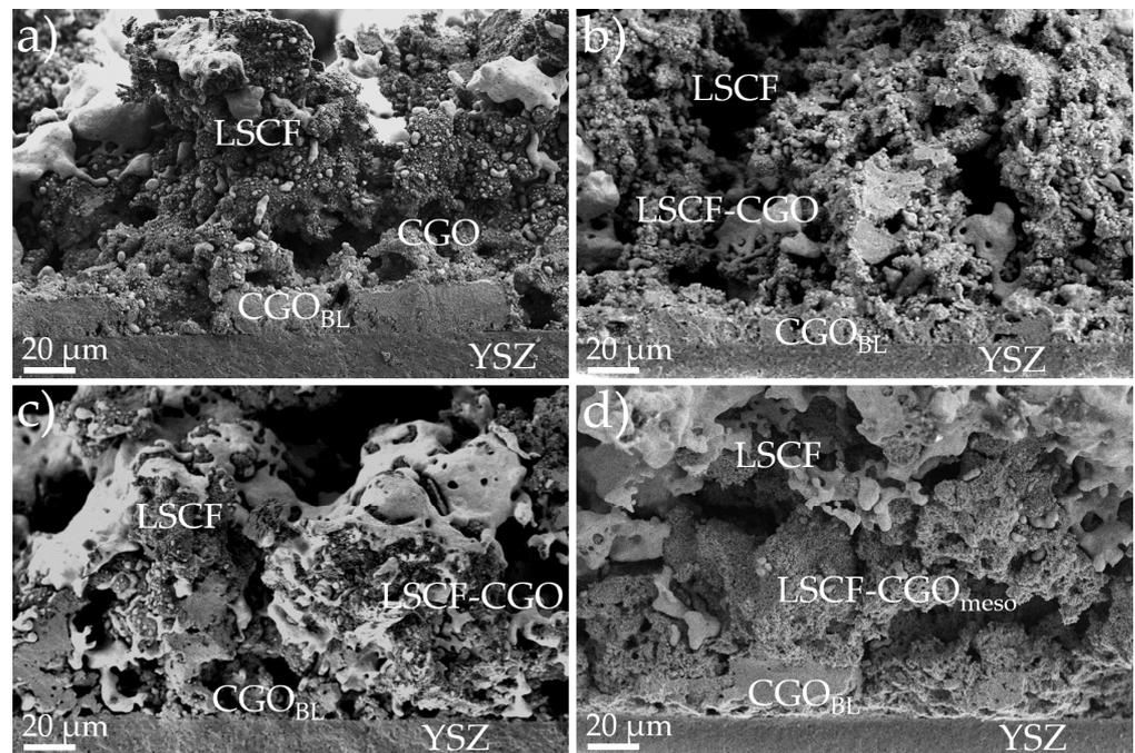
**Figure 3.** Cross-sectional SEM micrographs of the four different cells. (a) Micrograph of the CGO cell, fabricated with no infiltration. (b) Micrograph of the cell fabricated with slow infiltration and 5/20 sat. (5-CGO). (c) Micrograph of the cell fabricated with fast infiltration and 10/20 sat. (10-CGO). (d) Micrograph of the cell fabricated with a mesoporous CGO scaffold and fast infiltration (10-CGO<sub>meso</sub>).
