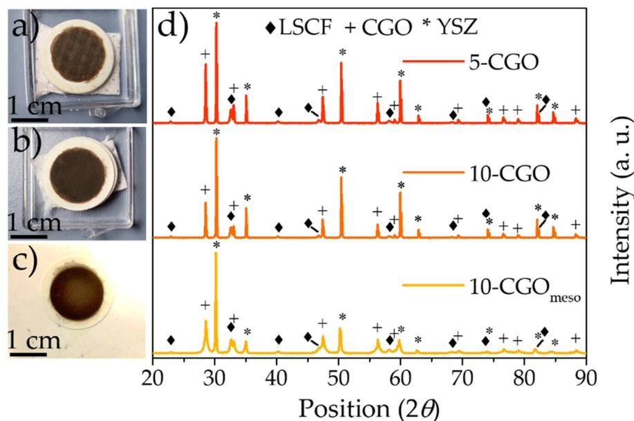
**Figure 2.** Digital pictures of the 5-CGO (a), 10-CGO (b) and 10-CGO<sub>meso</sub> (c) cells. XRD of the 5-CGO, 10-CGO and 10-CGO<sub>meso</sub> cells after the infiltration and calcination of the LSCF solution (d). The presence of the LSCF characteristic peaks confirms the formation of the perovskite after the calcination process.
