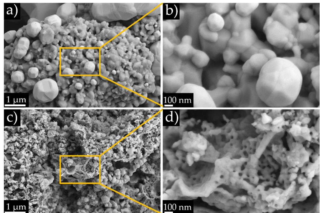
**Figure 4.** Representative region of the scaffold of the 10-CGO cell (a). SEM micrograph at a higher magnification (b). Representative region of the infiltrated scaffold of the 10-CGO<sub>meso</sub> cell (c). SEM micrograph at a higher magnification (d) where the residual mesoporosity can be observed.
