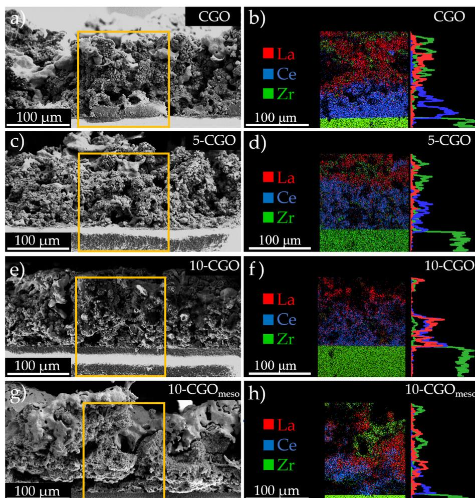
**Figure 5.** Representative SEM micrographs and EDX elemental maps of the CGO cell (panels (a,b)), the 5-CGO cell (panels (c,d)), the 10-CGO cell (panels (e,f)) and the 10-CGO<sub>meso</sub> cell (panels (g,h)). In all the EDX maps, the YSZ, CGO and LSCF phases are indicated by their main representative element. Zr (green), Ce (blue) and La (red) show the presence of YSZ, CGO and LSCF, respectively.
