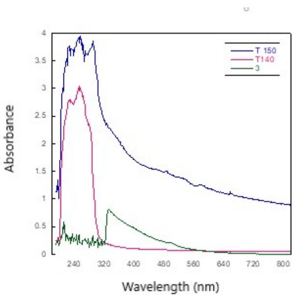
**Figure S1.** The UV absorption spectra of the w-ZnS powder washing solutions: w-ZnS produced at 150°C (blue), at 140°C (red) and of clean solvent (green).
