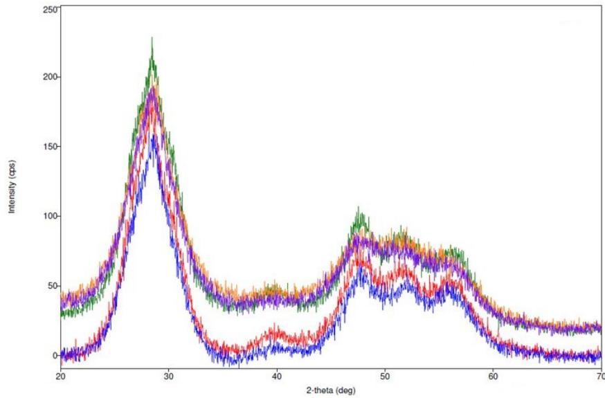
**Figure S1.** XRD diffractogram taken from the ZnS “standard” samples – red and blue, and from the “recycled” samples – green, orange and purple lines.
