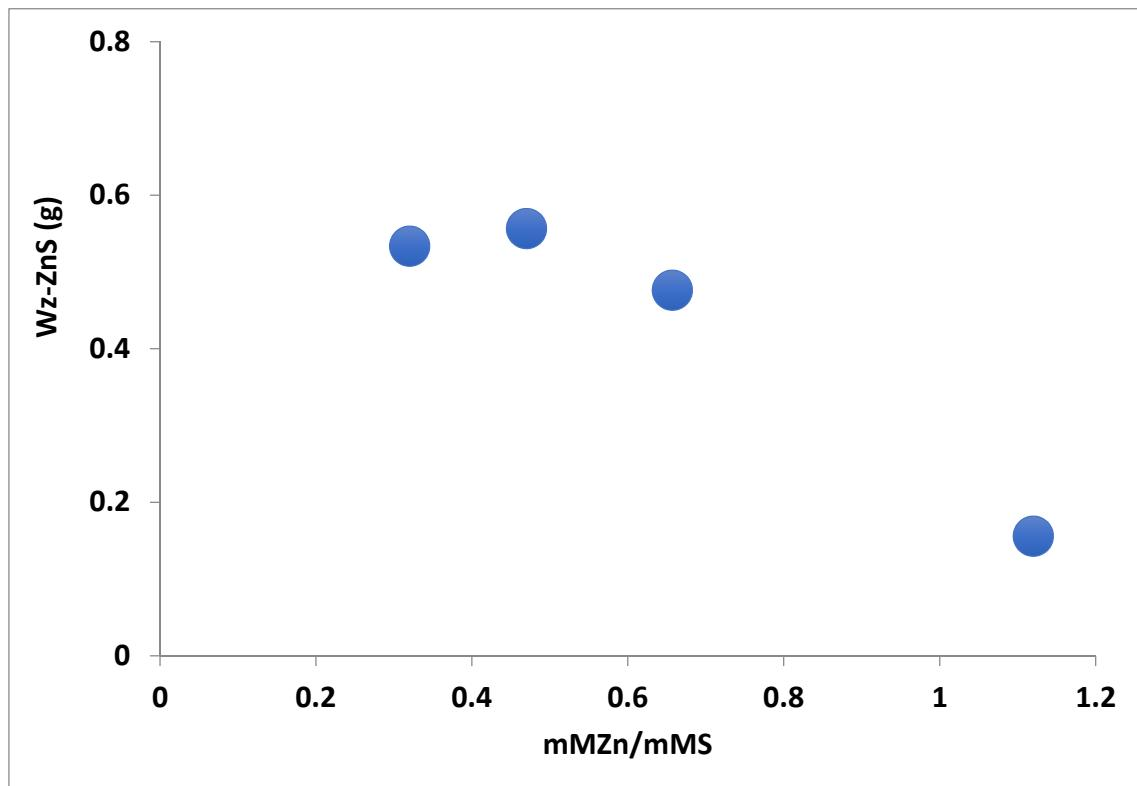
**Figure S2.** The graph showing the production of w-ZnS (in grammes) as a function of the nmZn/nMS molar ratio used in the synthesis.
