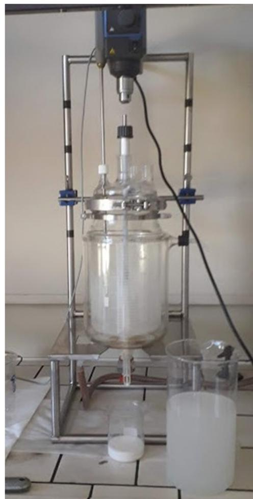
**Figure S4.** The glass reactor of the pilot plant and jars containing the recycled solvent (right) and the w-ZnS solution (left). The pilot plant consists of a 5 L transparent jacketed glass reactor with the mechanical stirrer,
