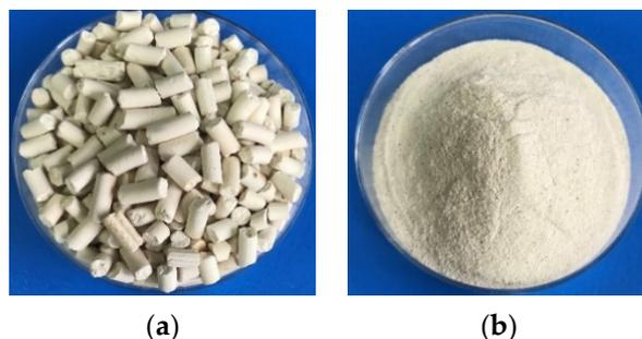
**Figure 2.** Images of: (a) 13X zeolite in pellets form; (b) powder of 13X zeolite.
