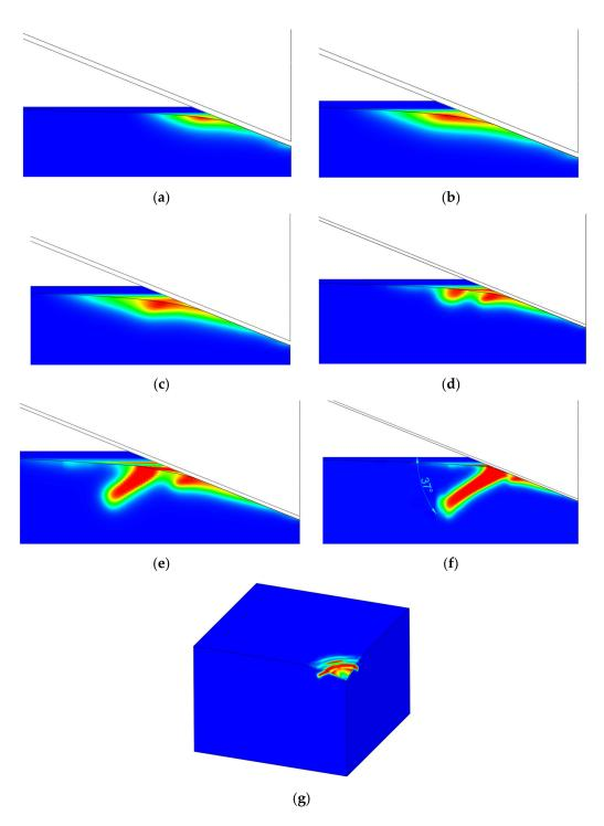
**Figure 8.** Stable crack growth with inclination angle at different penetration depths: (a)  $u = 1.2 \mu m$ , (b)  $u = 1.65 \mu m$ , (c)  $u = 2.025 \mu m$ , (d)  $u = 2.4 \mu m$ , (e)  $u = 2.8 \mu m$ , (f)  $u = 3.375 \mu m$ , front view for different penetration depths, and (g) isometric view without indenter at  $u = 3.375 \mu m$  (max. loading).
