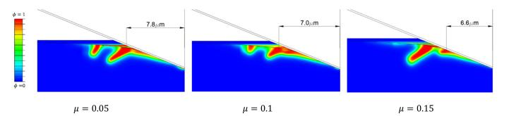
**Figure 6.** Comparison of the crack growth for different values of the friction coefficient,  $\mu$ . All deformed models are under the same indenter penetration, i.e.,  $h = 3 \mu m$ .
