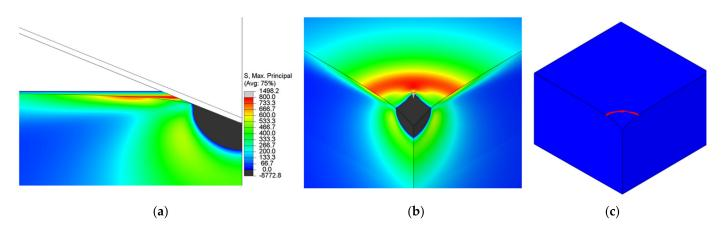
**Figure 7.** Positive maximum principal stress (in MPa) on specimen surface as a cause of cone-crack initiation, (**a**) stress distribution (in MPa) in front plane, (**b**) stress distribution in isometric view (without the indenter), showing ring-like distribution outside the contact region, and (**c**) isometric view (without the indenter) of the initiation ring.
