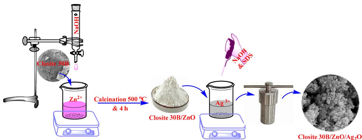
**Figure 1.** Schematic view of Cloisite 30B/ZnO/Ag<sub>2</sub>O photocatalyst synthesis process.
